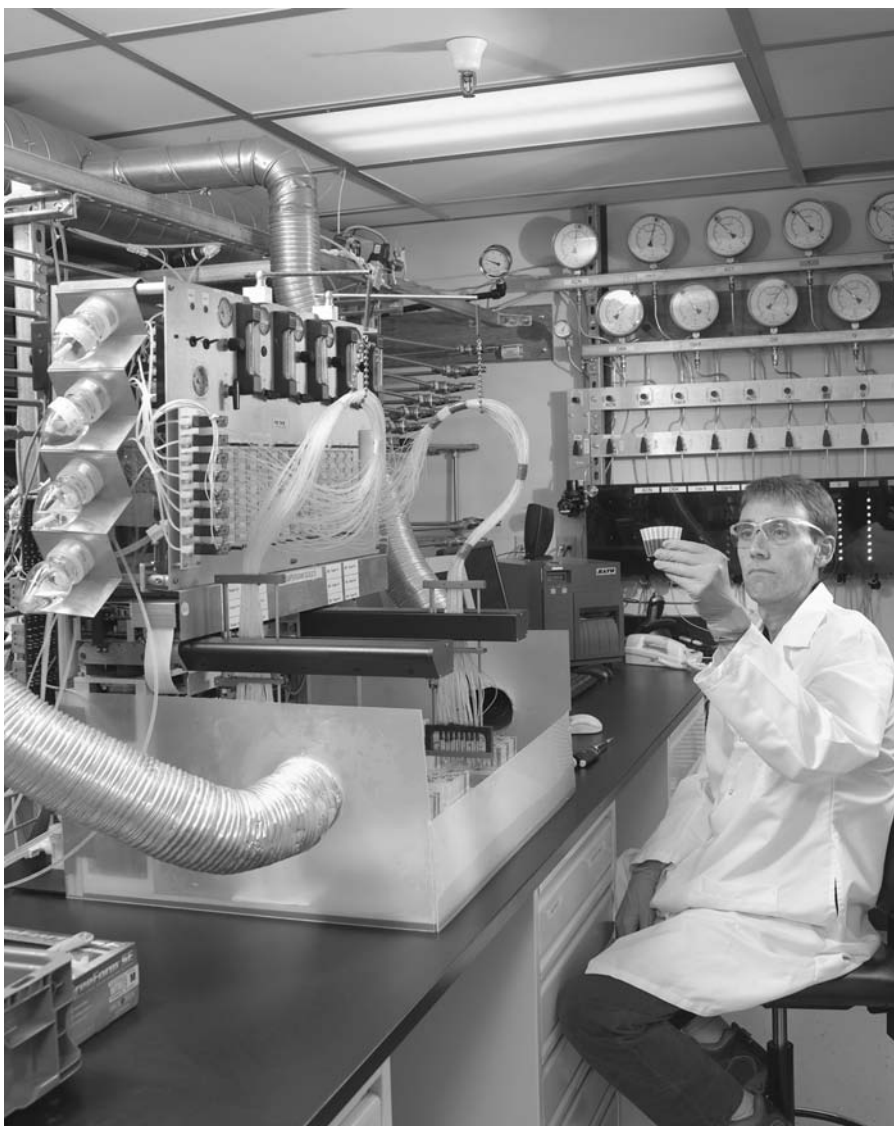
Figure 5–2. David Seebach, oligo technician, operating the SuperSAM™ high-throughput DNA synthesizer. See Color Plates.
