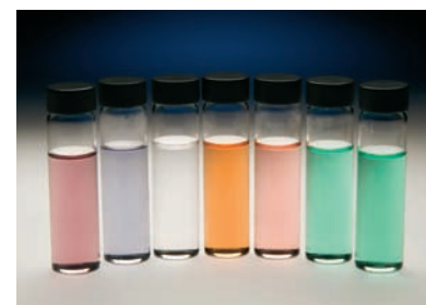
Figure 22.16 Colors of some of the first-row transition metal ions in solution. From left to right: \text{Ti}^{3+} , \text{Cr}^{3+} , \text{Mn}^{2+} , \text{Fe}^{3+} , \text{Co}^{2+} , \text{Ni}^{2+} , \text{Cu}^{2+} . The \text{Sc}^{3+} and \text{V}^{5+} ions are colorless.
