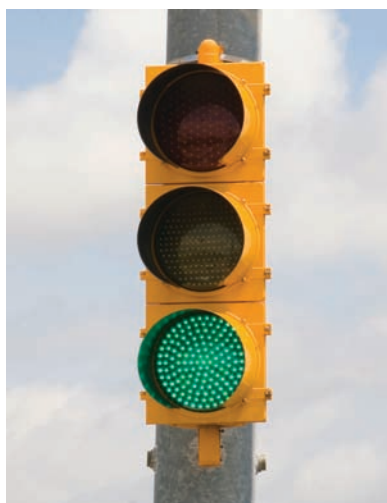
Figure 25.17 LED arrays in traffic signals. Many communities have replaced the red and green signals with LED arrays that are much more energy efficient than the incandescent bulbs used previously. The yellow lights are being replaced more slowly, however, because LED arrays are expensive and the short duration of yellow lights would not necessarily allow an overall cost saving when the energy efficiency is factored in.
