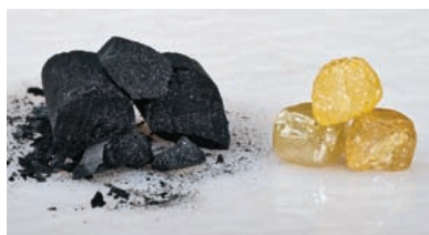
Figure 24.5 A synthetic diamond and the starting material—graphite.
