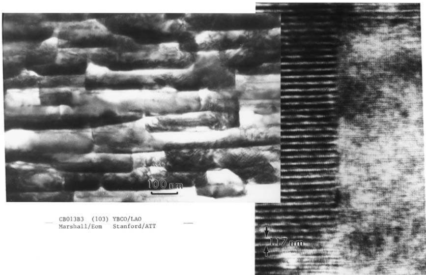
Fig. 12.13. Low and high magnification of a plan-view (103) film tilted 45° about the [010] axis. At low magnification it is observed that the grain boundaries are in the twist orientation (normal to [010]) whereas on a finer microscopic scale at high magnification it is observed that the boundaries may be faceted.
