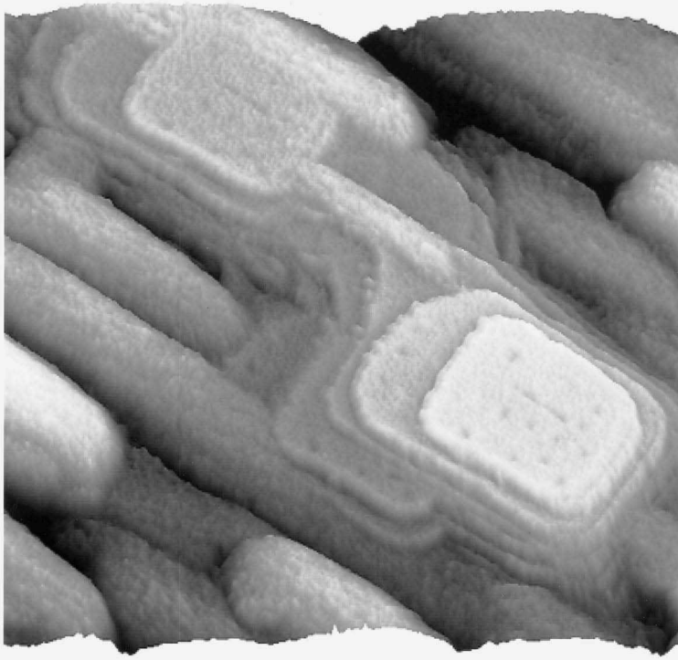
Fig. 6.14. The STM captured the beginning of a -axis growth on the underlying c -axis material in this image of YBCO grown on NdGaO 3 .
