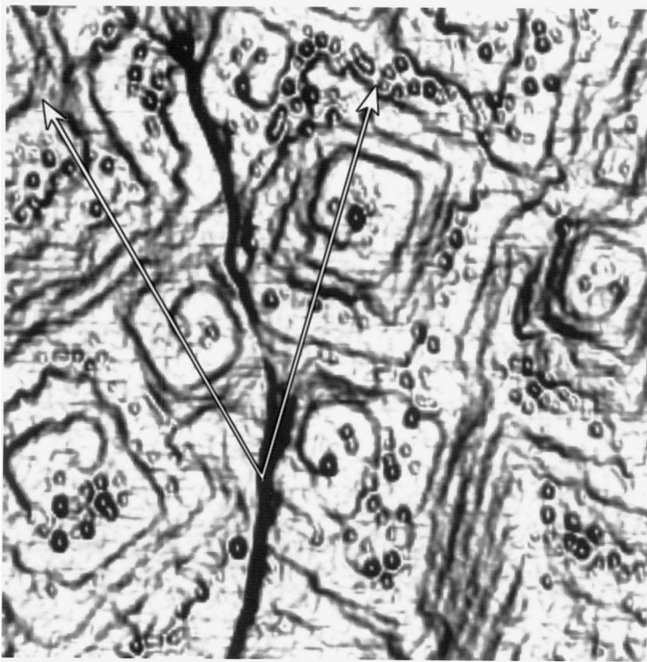
Fig. 6.19. A higher-resolution AFM image of one of the SrTiO 3 bicrystal YBCO junctions in Fig. 6.18 showing the 36.8° rotation of spiral grains across the junction.
