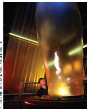
Polyethylene films are produced by extruding the molten plastic through a ring-like gap and inflating the film into a balloon.
