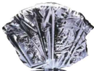
▲ Figure 7.18 Elemental silicon, which is a metalloid. Although it looks metallic, silicon is brittle and is a poor thermal and electrical conductor compared to metals. Large crystals of silicon are sliced into thin wafers for use in integrated circuits.
