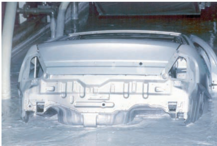
► Figure 18.21 An automobile body receives a corrosion protection coating containing yttrium in place of lead.
