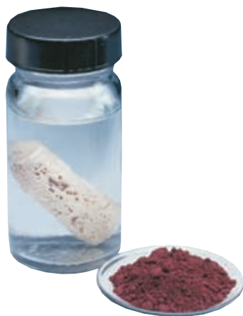
▲ Figure 22.39 White and red allotropes of phosphorus. White phosphorus is very reactive and is normally stored under water to protect it from oxygen. Red phosphorus is much less reactive than white phosphorus, and it is not necessary to store it under water.
