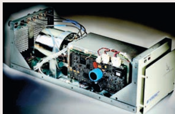
▲ Figure 12.30 A view of the amplifier employing a superconducting filter to receive cell phone signals. The cylindrical object to the left is the cryogenic refrigerator used to keep the filter at a temperature below its T_c value.
