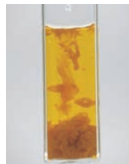
► Figure 23.30 Addition of a NaOH solution to an aqueous solution of \text{Fe}^{3+} causes \text{Fe}(\text{OH})_3 to precipitate.
