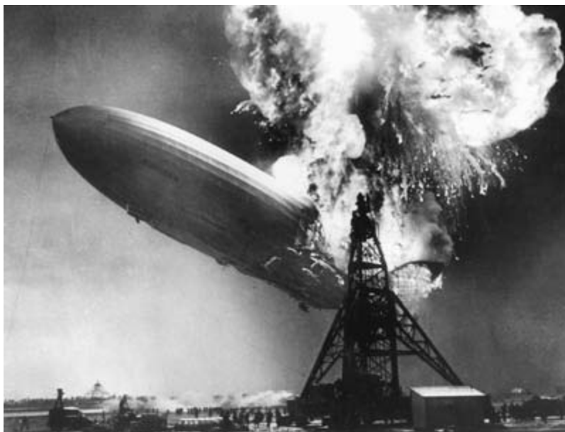
◀ Figure 5.15 The burning of the hydrogen-filled airship Hindenburg in Lakehurst, New Jersey, on May 6, 1937. This photo was taken only 22 seconds after the first explosion occurred. This tragedy led to the discontinuation of hydrogen as a buoyant gas in such craft. Modern-day blimps are filled with helium, which is not as buoyant as hydrogen, but is not flammable.
