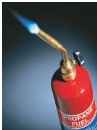
▲ Figure 3.7 Propane, C 3 H 8 , burns in air, producing a blue flame. The liquid propane vaporizes and mixes with air as it escapes through the nozzle.
