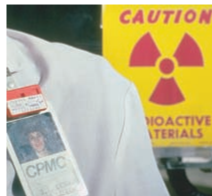
▲ Figure 21.9 Badge dosimeter. Badges such as the one on this worker's lapel are used to monitor the extent to which the individual has been exposed to high-energy radiation. The radiation dose is determined from the extent of fogging of the film in the dosimeter. Monitoring the radiation in this way helps prevent overexposure for people whose jobs require them to use radioactive materials or X rays.
