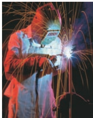
▲ Figure 22.17 Welding with an oxyacetylene torch. The heat of combustion of acetylene is exceptionally high, thus giving rise to a very high flame temperature.
