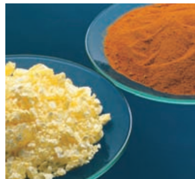
▲ Figure 2.25 Compounds of ions of the same element but with different charge can be very different in appearance. Both substances shown are complex salts of iron with \text{K}^+ and \text{CN}^- ions. The one on the left is potassium ferrocyanide, which contains Fe(II) bound to \text{CN}^- ions. The one on the right is potassium ferricyanide, which contains Fe(III) bound to \text{CN}^- ions. Both substances are used extensively in blueprinting and other dyeing processes.
