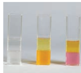
▲ Figure 22.9 Aqueous solutions of NaF, NaBr, and NaI (from left to right) to which Cl 2 has been added. Each solution is in contact with carbon tetrachloride (CCl 4 ), which forms the lower layer in each container. The halogens are more soluble in CCl 4 than in H 2 O. The F - ion in the NaF solution (left) does not react with Cl 2 ; both the aqueous and CCl 4 layers remain colorless. The Br - ion (center) is oxidized by Cl 2 to form Br 2 , producing a yellow aqueous layer and an orange CCl 4 layer. The I - ion (right) is oxidized to I 2 , producing an amber aqueous layer and a violet CCl 4 layer.
