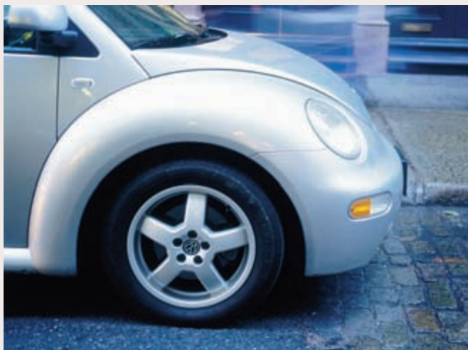
▲ Figure 12.15 The fenders of this New Beetle are made of General Electric Noryl GTX, a composite of nylon and polyphenylene ether.
