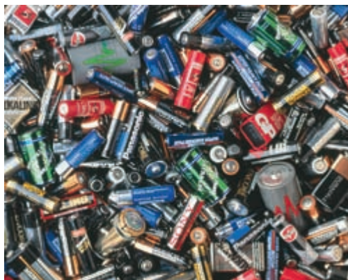
▲ Figure 20.19 Batteries are voltaic cells that serve as portable sources of electricity. Batteries vary markedly in size and in the electrochemical reaction used to generate electricity.
