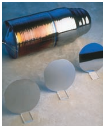
▲ Figure 22.49 Elemental silicon. To prepare electronic devices, silicon powder is melted, drawn into a single crystal, (top) by zone refining. Wafers of silicon (bottom), cut from the crystal, are subsequently treated by a series of elegant techniques to produce various electronic devices.
