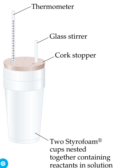
Figure 5.18 Coffee-cup calorimeter, in which reactions occur at constant pressure.
