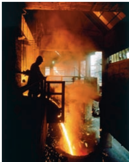
▲ Figure 6.5 The color and intensity of light emitted by a hot object depends on the temperature of the object. The temperature is highest at the center of this pour of molten steel. As a result, the light emitted from the center is most intense and of shortest wavelength.
