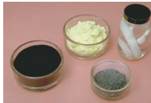
▲ Figure 7.16 Nonmetals are diverse in their appearances. Shown here are (clockwise from left) carbon as graphite, sulfur, white phosphorus (stored under water), and iodine.
