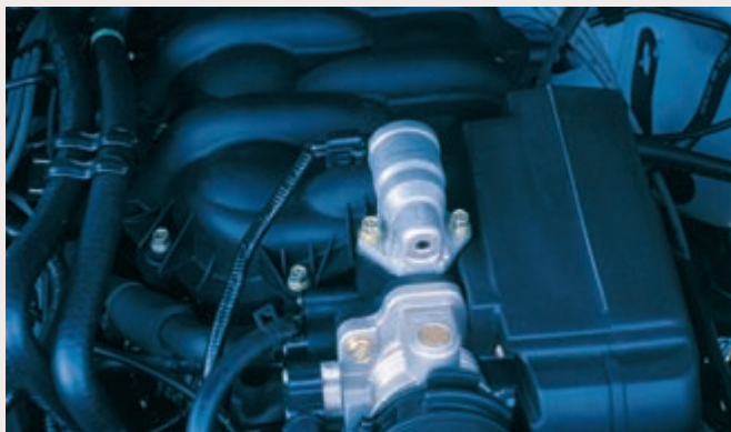
▲ Figure 12.14 The intake manifold for a series of Ford Motor Company V-8 engines is formed from nylon.
