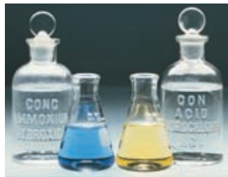
▲ Figure 4.7 The acid-base indicator bromthymol blue is blue in basic solution and yellow in acidic solution. The left flask shows the indicator in the presence of a base, aqueous ammonia (here labeled as ammonium hydroxide). The right flask shows the indicator in the presence of hydrochloric acid, \text{HCl} .
