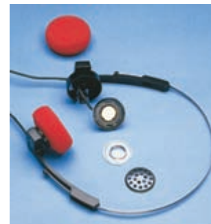
▲ Figure 23.19 Interior of a lightweight audio headset. The assembly can be made small because of the very strong magnetism of the \text{Co}_5\text{Sm} alloy used.
