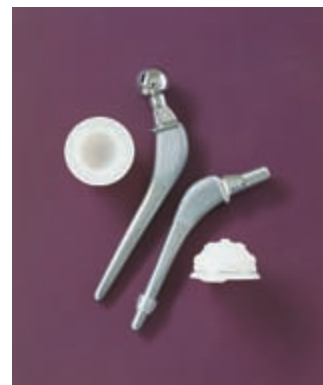
▲ Figure 12.22 The components of a modern hip-joint replacement. The metal ball is composed of a corrosion-resistant alloy. The cup, which receives the ball, is lined with high molecular weight polyethylene.
