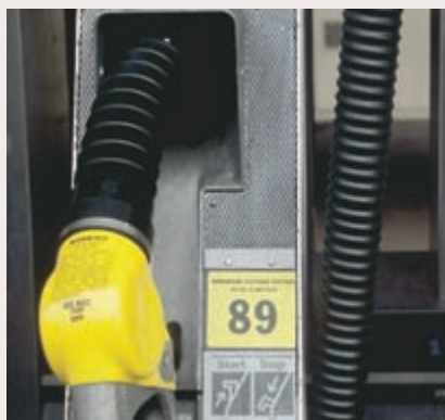
◀ Figure 25.8 The octane rating of gasoline measures its resistance to knocking when burned in an engine. The octane rating of this gasoline is 89, as shown on the face of the pump.
