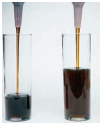
▲ Figure 11.13 The Society of Automotive Engineers (SAE) has established numbers to indicate the viscosity of motor oils. The higher the number, the greater the viscosity at any given temperature. The SAE 40 motor oil on the left is more viscous and flows more slowly than the less viscous SAE 10 oil on the right.
