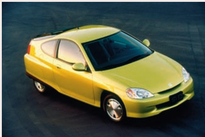
▲ Figure 5.25 The Honda Insight, a hybrid car in which both batteries and a gasoline engine provide power to move the car, as well as drive ancillary devices.
