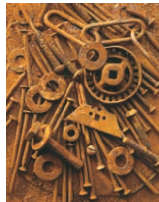
▲ Figure 20.24 Corrosion of iron in a shipyard. The corrosion of iron is an electrochemical process of great economic importance. The annual cost of metallic corrosion in the United States is estimated to be $70 billion.
