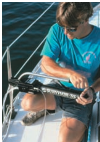
▲ Figure 18.15 This hand-operated water desalinator works by reverse osmosis. It can produce 4.5 L (1.2 gal) of pure water from seawater in an hour.
