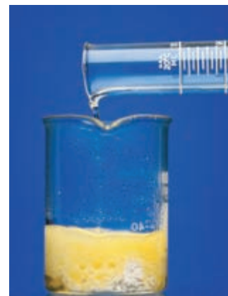
▲ Figure 22.46 Solid \text{CaCO}_3 reacts with a solution of hydrochloric acid to produce \text{CO}_2 gas, seen here as the bubbles in the beaker.
