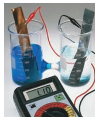
▲ Figure 20.4 A voltaic cell based on the reaction in Equation 20.7. The left compartment contains 1 M \text{CuSO}_4 and a copper electrode. The one on the right contains 1 M \text{ZnSO}_4 and a zinc electrode. The solutions are connected by a porous glass disc, which permits contact of the two solutions. The metal electrodes are connected through a voltmeter, which reads the potential of the cell, 1.10 V.
