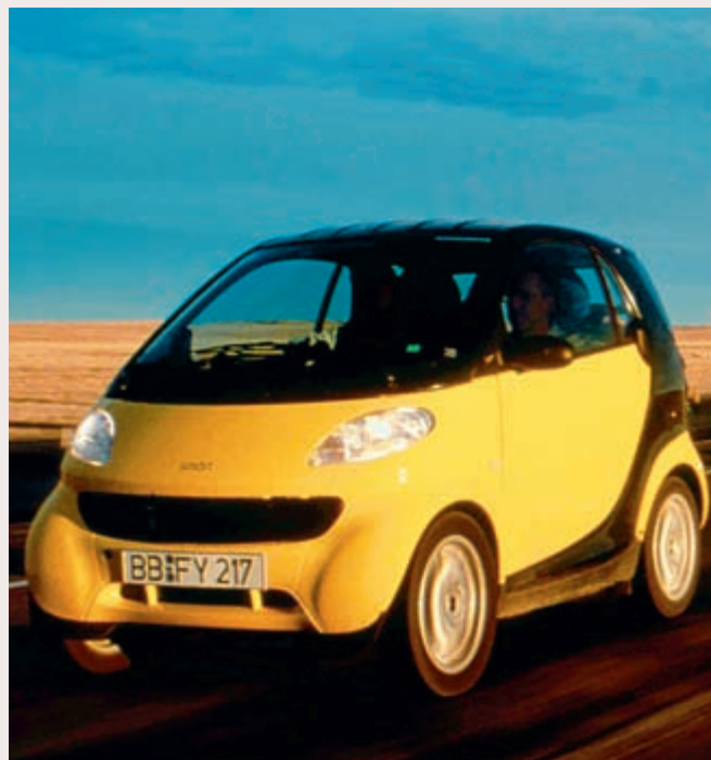
▲ Figure 12.16 This experimental car has body panels that are made of a polycarbonate-polybutylene plastic.
