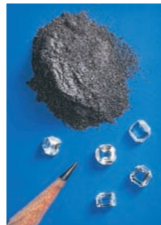
▲ Figure 22.44 Graphite and a synthetic diamond prepared from graphite. Most synthetic diamonds lack the size, color, and clarity of natural diamonds and are therefore not used in jewelry.
