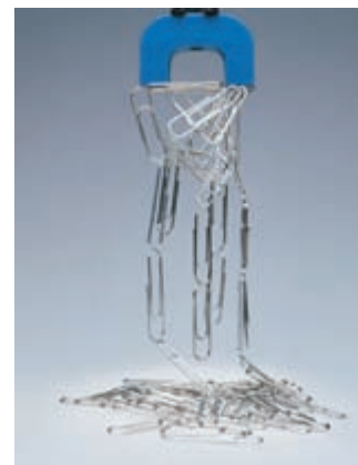
▲ Figure 23.26 Permanent magnets are made from ferromagnetic materials.
