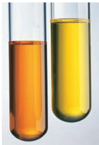
▲ Figure 23.28 Sodium chromate, \text{Na}_2\text{CrO}_4 (on the right), and potassium dichromate, \text{K}_2\text{Cr}_2\text{O}_7 (on the left), illustrate the difference in color of the chromate and dichromate ions.
