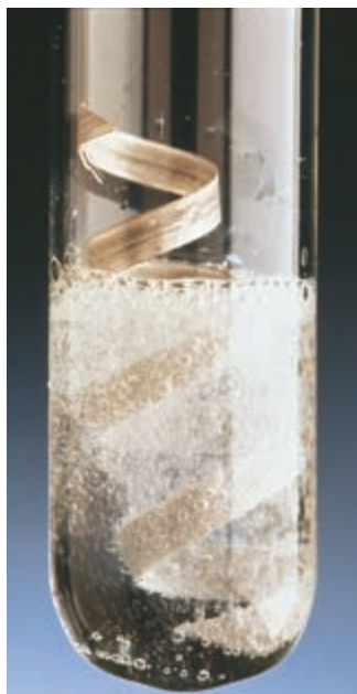
▲ Figure 4.13 Many metals, such as the magnesium shown here, react with acids to form hydrogen gas. The bubbles are due to the hydrogen gas.
