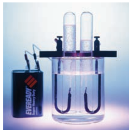
▲ Figure 1.7 Water decomposes into its component elements, hydrogen and oxygen, when a direct electrical current is passed through it. The volume of hydrogen (on the right) is twice the volume of oxygen (on the left).
