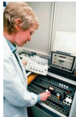
▲ Figure 21.11 A scintillation counter, used to quantitatively measure the level of radiation.
