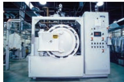
▲ Figure 18.20 This dry-cleaning apparatus employs supercritical \text{CO}_2 as solvent.
