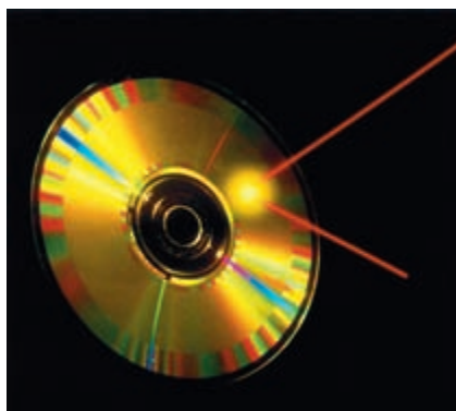
▲ Figure 6.9 A laser beam reflected from surface of a CD disk. CD players and similar devices use a small laser beam to read the information on the disk.
