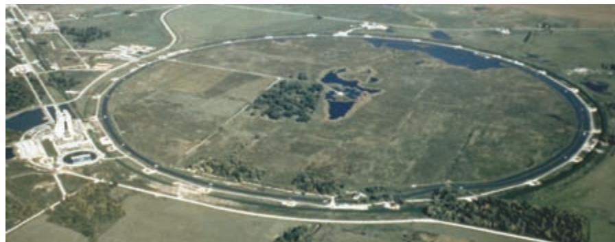
◀ Figure 21.6 An aerial view of the Fermi National Accelerator Laboratory at Batavia, Illinois. Particles are accelerated to very high energies by circulating them through magnets in the ring, which has a circumference of 6.3 km.
