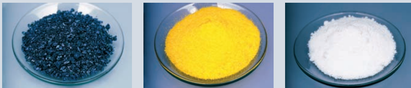
▲ Figure 24.37 From left to right, \text{KMnO}_4 , \text{K}_2\text{CrO}_4 , and \text{KClO}_4 . \text{KMnO}_4 and \text{K}_2\text{CrO}_4 are intensely colored due to ligand-to-metal charge transfer (LMCT) transitions in the \text{MnO}_4^- and \text{CrO}_4^{2-} anions. There are no valence d orbitals on Cl, so the charge-transfer transition for \text{ClO}_4^- requires ultraviolet light and \text{KClO}_4 is white.
