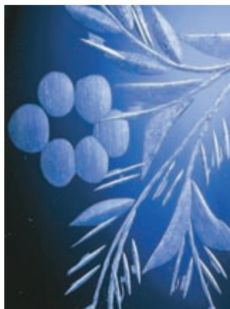
▲ Figure 22.13 Etched or frosted glass. Designs such as this are produced by first coating the glass with wax. The wax is then removed in the areas to be etched. When treated with hydrofluoric acid, the exposed areas of the glass are attacked, producing the etching effect.
