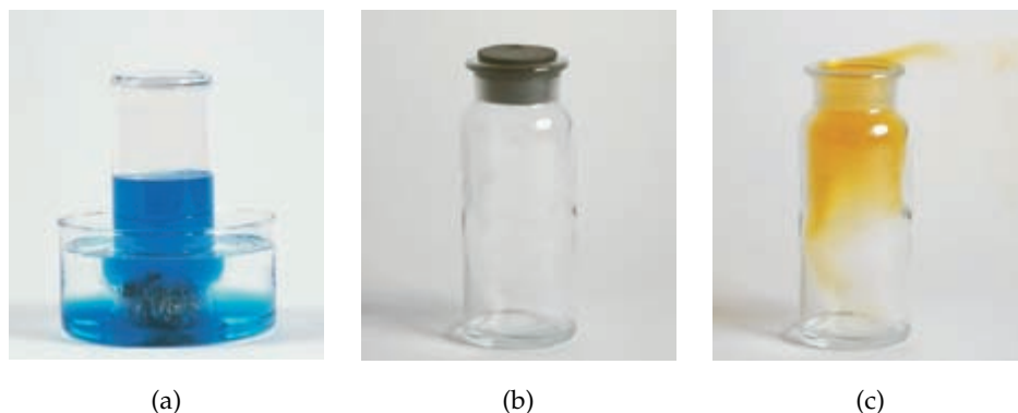
◀ Figure 22.33 (a) Nitric oxide (NO) can be prepared by the reaction of copper with 6 M nitric acid. In this photo a jar containing 6 M HNO 3 has been inverted over some pieces of copper. Colorless NO, which is only slightly soluble in water, is collected in the jar. The blue color of the solution is due to the presence of Cu 2+ ions. (b) Colorless NO gas, collected as shown on the left. (c) When the stopper is removed from the jar of NO, the NO reacts with oxygen in the air to form yellow-brown NO 2 .
