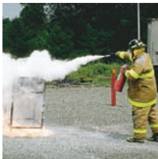
▲ Figure 10.14 The \text{CO}_2 gas from a fire extinguisher is denser than air. The \text{CO}_2 cools significantly as it emerges from the tank. Water vapor in the air is condensed by the cool \text{CO}_2 gas and forms a white fog accompanying the colorless \text{CO}_2 .
