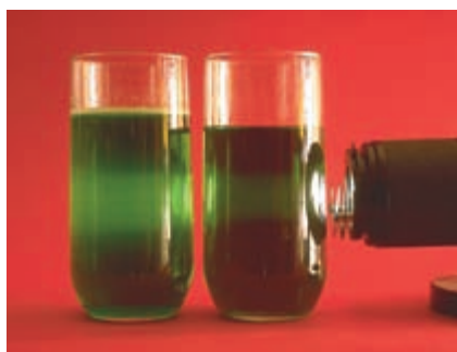
▲ Figure 13.27 Illustration of the Tyndall effect. The vessel on the left contains a colloidal suspension; that on the right, a solution. The path of the beam through the colloidal suspension is seen because the light is scattered by the colloidal particles. Light is not scattered by the individual solute molecules in the solution.
