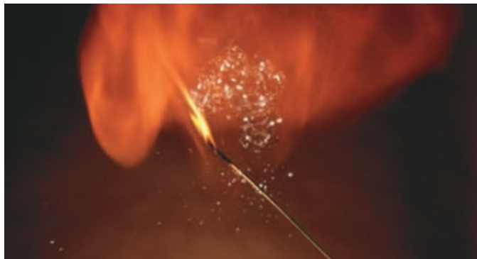
► Figure 3.2 Combustion of hydrogen gas. The gas is bubbled through a soap solution forming hydrogen-filled bubbles. As the bubbles float upwards, they are ignited by a candle on a long pole. The orange flame is due to the reaction of the hydrogen with oxygen in the air and results in the formation of water vapor.
