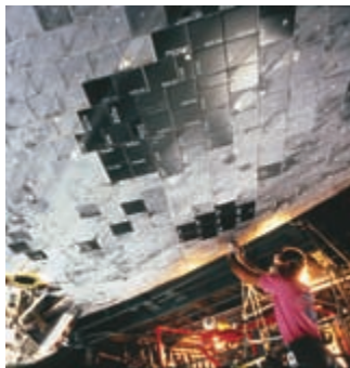
▲ Figure 12.25 A worker applying thermally insulating ceramic tiles to the body of the Space Shuttle orbiter.
