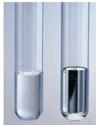
▲ Figure 11.16 The water meniscus in a glass tube compared with the mercury meniscus in a similar tube.
