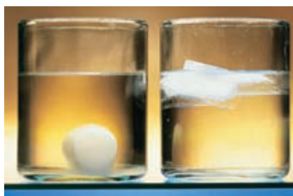
▲ Figure 11.9 As with most substances, the solid phase of paraffin is denser than the liquid phase, and the solid therefore sinks below the liquid surface (left). In contrast, the solid phase of water, ice, is less dense than its liquid phase (right) causing the ice to float on the water. Richard Megna/Fundamental Photographs.
