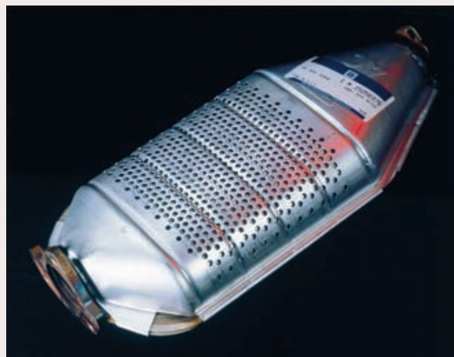
▲ Figure 14.22 A stainless steel catalytic converter used in automobiles. The converter contains catalysts that promote the conversion of exhaust gases into \text{CO}_2 , \text{H}_2\text{O} , and \text{N}_2 .
