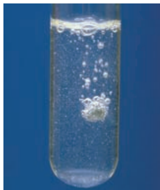
▲ Figure 7.25 Calcium metal reacts with water to form hydrogen gas and aqueous calcium hydroxide, \text{Ca}(\text{OH})_2(\text{aq}) .
