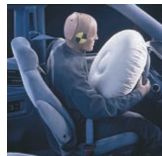
▲ Figure 3.6 The decomposition of sodium azide, NaN_3(s) , is used to inflate automobile air bags. When properly ignited, the NaN_3 decomposes rapidly, forming nitrogen gas, N_2(g) , which expands the air bag.
