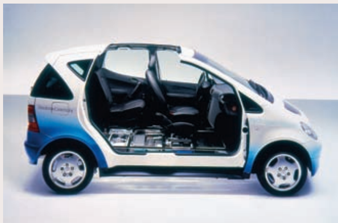
▲ Figure 1.21 Cutaway view of car powered by fuel cells.
