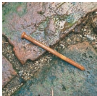
▲ Figure 19.9 The rusting of iron, such as this nail, is a spontaneous process. The reaction, Equation 19.4, leads to a decrease in the entropy of the system—that is, \Delta S_{\text{sys}} is negative. Nevertheless, the second law demands that \Delta S_{\text{univ}} must be positive, which means that \Delta S_{\text{surr}} is a positive number of greater magnitude than \Delta S_{\text{sys}} .
