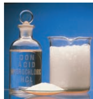
▲ Figure 4.9 Carbonates react with acids to form carbon dioxide gas. Here \text{NaHCO}_3 (white solid) reacts with hydrochloric acid; the bubbles contain \text{CO}_2 .
