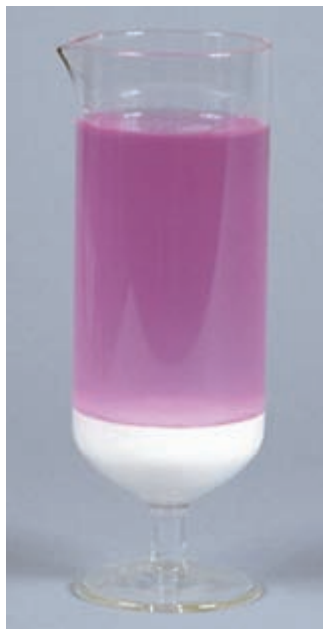
\blacktriangle Figure 22.20 Barium oxide ( \text{BaO} ), the white solid at the bottom of the container, reacts with water to produce barium hydroxide [ \text{Ba}(\text{OH})_2 ]. The reddish purple color of the solution is caused by phenolphthalein and indicates the presence of \text{OH}^- ions in solution.
