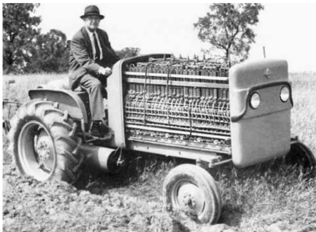
Fig. 1. Dr Harry Karl Ihrig driving the Allis-Chalmers’ fuel cell-powered tractor (Photo reproduced from W. Mitchell (Ed.), Fuel Cells , Academic Press, New York, 1963.)
