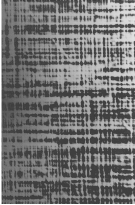
Figure 9.1 Double-crystal X-ray topograph of a heavily relaxed (001)-oriented GaAsSb layer on GaAs showing the characteristic 'tweed' contrast from two sets of misfit dislocations running parallel to the (110) directions
