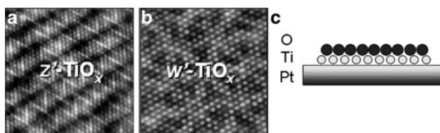
Fig. 14.1 STM images of the two different \text{TiO}_x/\text{Pt}(111) phases discussed in the present work. (a) z' phase, 9 \times 9 \text{ nm}^2 , V = 0.8 \text{ V} , I = 1.5 \text{ nA} . (b) w' phase, 6 \times 6 \text{ nm}^2 , V = 0.2 \text{ V} , I = 1.0 \text{ nA} . (c) Schematic drawing of the Pt/Ti/O stacking sequence. Adapted with permission from Ref. [38] Copyright 2005 by the American Chemical Society and Ref. [62] Copyright 2007 by the American Chemical Society
