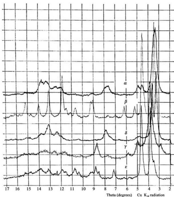
Fig. 8.2 X-ray diffraction patterns of five modifications of CuPc. (From Herbst and Hunger 1997, with permission.)
