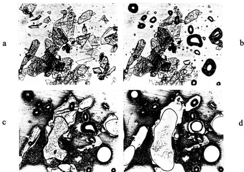
Fig. 4.2 Melting behaviour of sulphathiazole. (a) 175 °C, which is the melting point for commercially available Form II, (b) some Form II crystals melting at 175 °C, while others transform to the stable modification, (c) 200 °C, at which point some of the stable form begins to melt, (d) the equilibrium melting point (Kuhnert-Brandstätter 1971) for the higher melting form. (From Kuhnert-Brandstätter 1971, with permission.)
