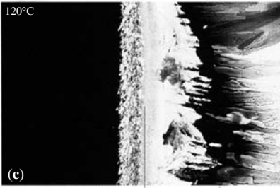
(c) Benzocaine Picric acid Eutectic Picric acid/BCPA 1:1 mod.II Peritectic BCPA 2:1/BCPA 1:1 mod.II
