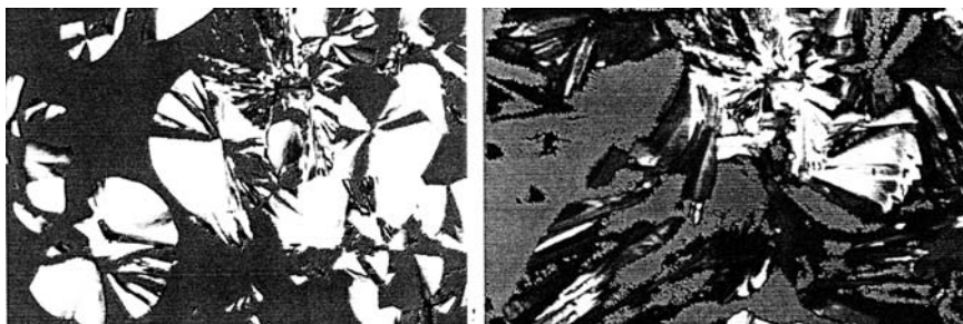
Fig. 4.11 Photomicrographs of sulphapyridine at two temperatures. Left, \sim 110^\circ\text{C} ; most of the field contains the metastable form that crystallized (peak B in Fig. 4.10). Right, \sim 180^\circ\text{C} (between peaks E and F in Fig. 4.11), most of the material has been converted to the stable form. (Reprinted from Schwarz and de Buhr 1998, with permission.)
