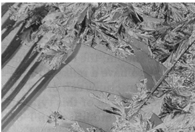
Fig. 4.4 (See also colour plate section.) Phase transformation of \beta -naphthol, showing the diffuse nature of product phase formation. (From Kuhnert-Brandstätter 1982, with permission.)
