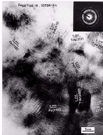
Fig. 6. The high-resolution transmission electron microscope (HR-TEM) observation of the shock consolidated Fe-63 vol. % TiN material at the pressure of 38.6 GPa. Structure was composed of the TiN and \alpha -Fe phases with the grain size of about 5 ~ 10 nm.
