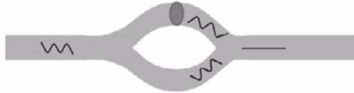
Fig. 33. Spin wave logic. The spin wave running through the two branches acquires a phase shift if it encounters 360^\circ a domain wall.
