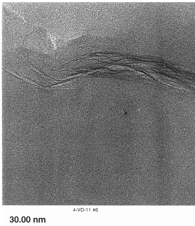
Figure 3.6 TEM of a disordered tactoid that would yield an X-ray pattern that would appear to be exfoliated.
