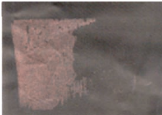
Figure 5. Adhesion (Scotch tape test) of PVDF/SLA1020 coating showing improved adhesion of graphite to copper current collector.
