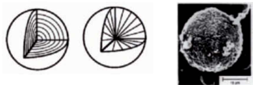
Figure 10. Depiction of the (a) Onion structure, the (b) Radial structure, and (c) Actual product MCMB, [16].
