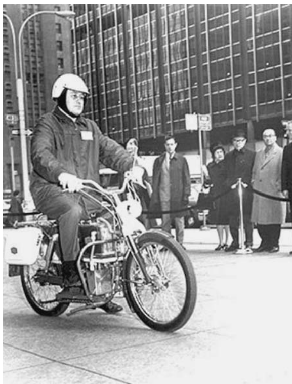
FIGURE 6.1 Karl Kordesch rides his hydrazine fuel cell motorcycle, 1967. (From Smithsonian Institution, neg. EMP059006, from the Science Service Historical Images Collection, courtesy of Union Carbide Corp.)
