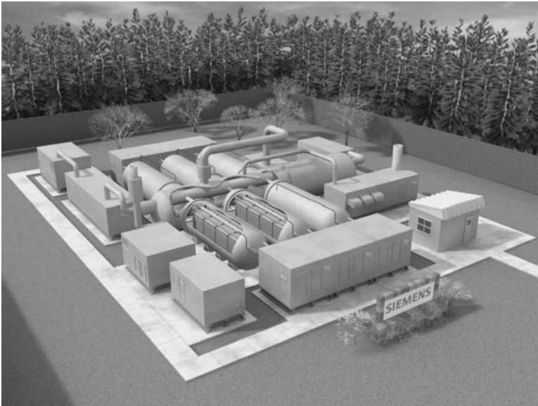
FIGURE 16.3 Overall view of a 3-MW SOFC-based Siemens–Westinghouse power station. (Courtesy of Siemens.)
