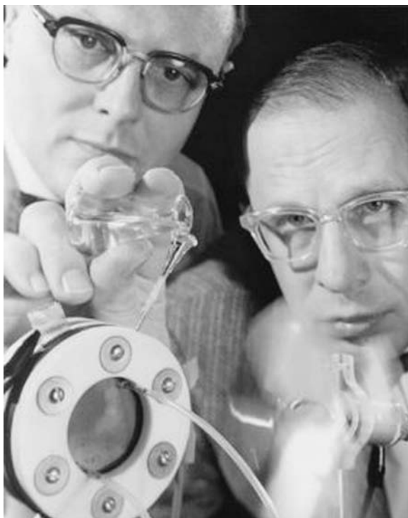
FIGURE 2.6 GE's Thomas Grubb (left) and Leonard Niedrach run a fan with a hydrocarbon-fed PEMFC, April 1963. (From Smithsonian Institution, neg. EMP059029, from the Science Service Historical Images Collection, courtesy of General Electric.)
