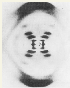
Fig. 9.26 The X-ray diffraction pattern obtained from a fibre of B-DNA. The black dots are the reflections, the points of maximum constructive interference, that are used to determine the structure of the molecule. (Adapted from an illustration that appears in J.P. Glusker and K.N. Trueblood, Crystal structure analysis: a primer . Oxford University Press (1972).)
