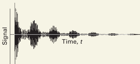
Fig. 12.34 A free-induction decay signal of a sample of ethanol. Its Fourier transform is the frequency-domain spectrum shown in Fig. 12.6. The total length of the image corresponds to about 1 s.
