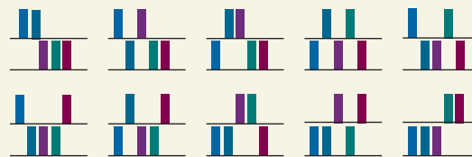
Fig. 13.1 Whereas a configuration \{5, 0, 0, \dots\} can be achieved in only one way, a configuration \{3, 2, 0, \dots\} can be achieved in the ten different ways shown here, where the tinted blocks represent different molecules.
