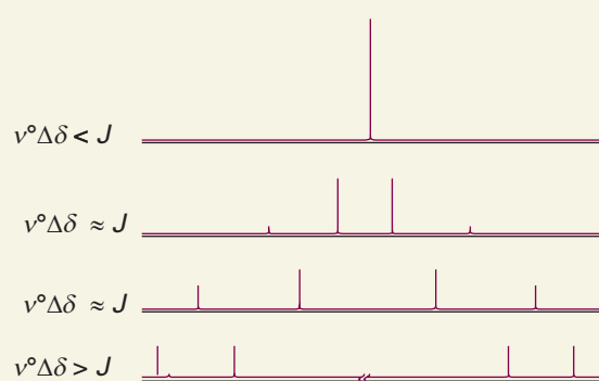
Fig. 12.26 The NMR spectra of an A_2 system (top) and an AX system (bottom) are simple ‘first-order’ spectra. At intermediate relative values of the chemical shift difference and the spin–spin coupling, complex ‘strongly coupled’ spectra are obtained. Note how the inner two lines of the bottom spectrum move together, grow in intensity, and form the single central line of the top spectrum. The two outer lines diminish in intensity and are absent in the top spectrum.
