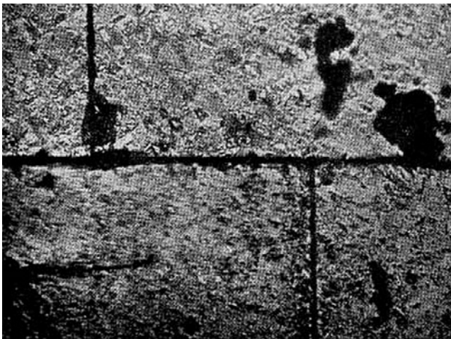
Figure 4.5-64 Grain boundary sliding on a bi-crystal tin (after Puttick and King, 1952; courtesy of Institute of Materials, Minerals and Mining).
