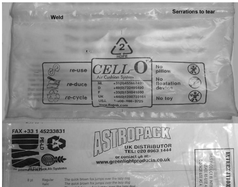
Figure 7.1-11 LDPE and HDPE macro-bubbles (deflated) on top of a test page with a range of font sizes.
