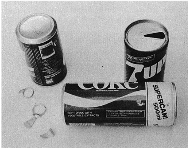
Figure 4.1-5 The aluminium drink can is an innovative product. The body is made from a single slug of a 3000 series aluminium alloy. The can top is a separate pressing which is fastened to the body by a rolled seam once the can has been filled. There are limits to one-piece construction.
