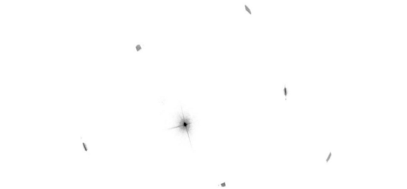
Figure 7.1-10 Diffraction pattern from a laser pointer, when shown on the track near the end of a music CD; the direct reflection has the cross pattern.
