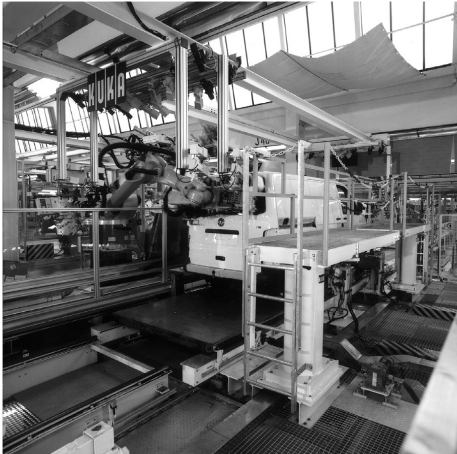
Figure 12.1-4 Joining allows the use of fundamentally dissimilar materials to achieve special function. Here a glass windshield consisting of glass mounted in a metal frame and sealed with a polymer is being robotically assembled into a modern automobile constructed of metal, plastic, or reinforced plastic. (Courtesy of KUKA Schweissanlagen GmbH, Augsburg, Germany, with permission.)
