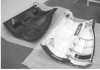
Figure 12.1-7 An adhesively bonded composite main landing gear door for an E2C (left) dramatically reduces part count, assembly labor, and weight compared to a conventional built-up, riveted Al-alloy door (right) for the same aircraft. (Courtesy of Northrop Grumman Corporation, El Segundo, CA, with permission.)
