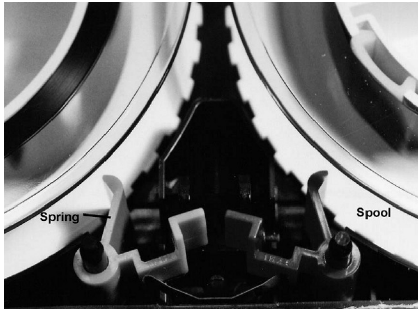
Figure 7.1-3 Mechanism that locks the spools when the tape is not being played, as seen inside a video cassette.
