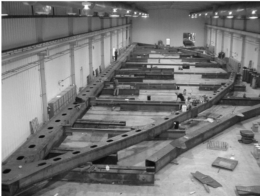
Figure 12.1-8 Sometimes joining is necessary not only because it allows something too large or too complicated to be created from one piece to be made, but also because the structure has to be constructed or erected on site, as is clearly the case for the bolted bridge shown. In modern bridge building, pre-fabricated details are joined on site after being pre-fitted in the more controlled environment of a fabrication shop (Courtesy of the American Bridge Company, Coraopolis, PA, with permission.)
