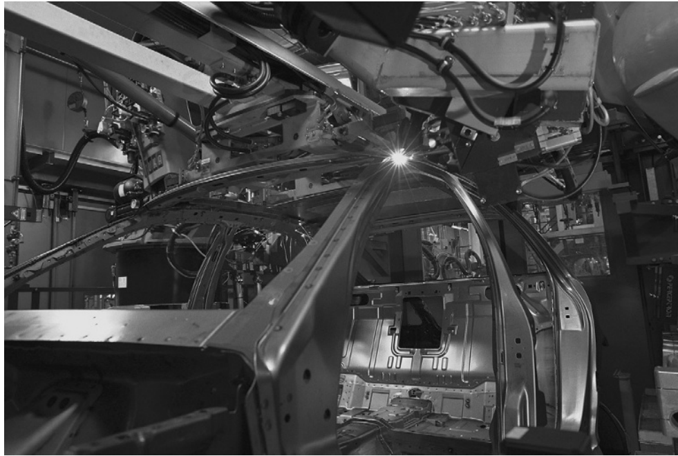
Figure 12.1-9 Modern manufacturing often benefits when labor-intensive, quality-critical assembly is automated, as exemplified in the automobile industry by robotic welding. (Courtesy of DaimlerChrysler AG, Stuttgart, Germany, with permission.)
