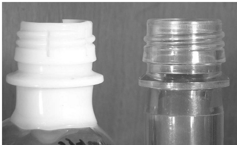
Figure 7.1-17 Details of the neck region of an injection-blow moulded PET bottle. The bottle on the left has been heat treated at 120 °C, while the neck of a preform is shown on the right.
