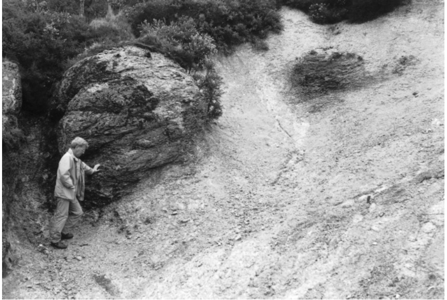
Fig. 4.15 Highly weathered granite, showing residual materials—mainly kaolinitized feldspar and quartz. The granite has broken down principally due to the weathering of feldspars. Note the ‘corestone’ of less weathered granite by the figure. Two Bridges Quarry, Dartmoor, UK. Photograph courtesy of J. Andrews.
