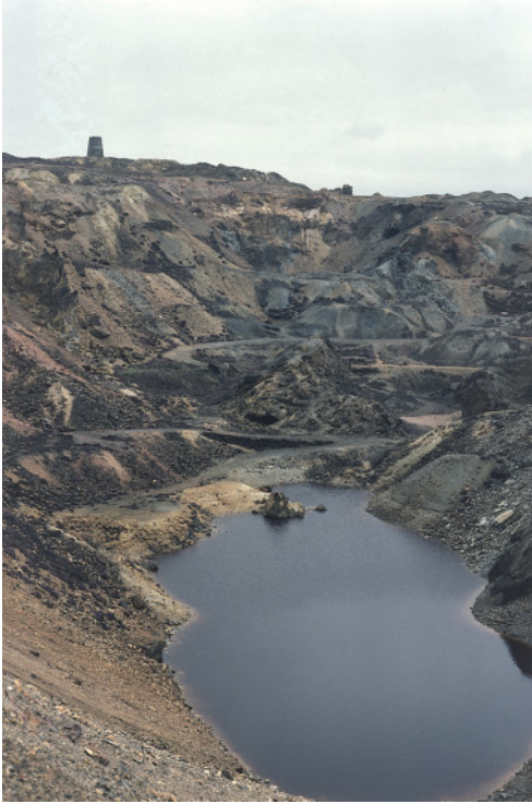
Plate 5.1 Excavations for copper at Parys Mountain, Anglesey, UK. The spoil heaps provide a huge surface area for sulphide oxidation. The lake waters in the pit bottom have pH below 3. Photograph courtesy of J. Andrews.
