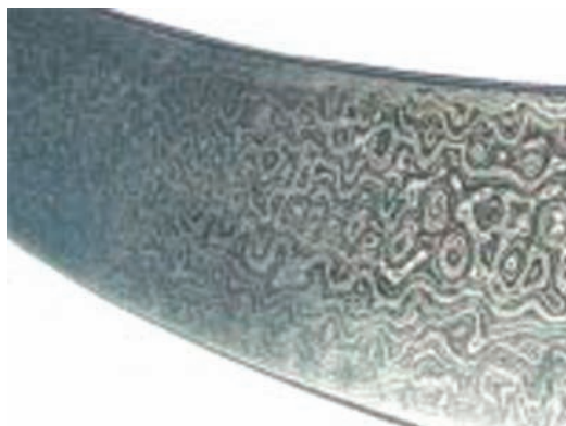
Figure 1.5 Typical wavy patterns on the surface of a Damascus saber. The structure was found to be due to carbon nanotubes in the saber alloy. (Reproduced with kind permission from Levin et al. , ref. 19. Copyright Wiley-VCH, 2005.)
