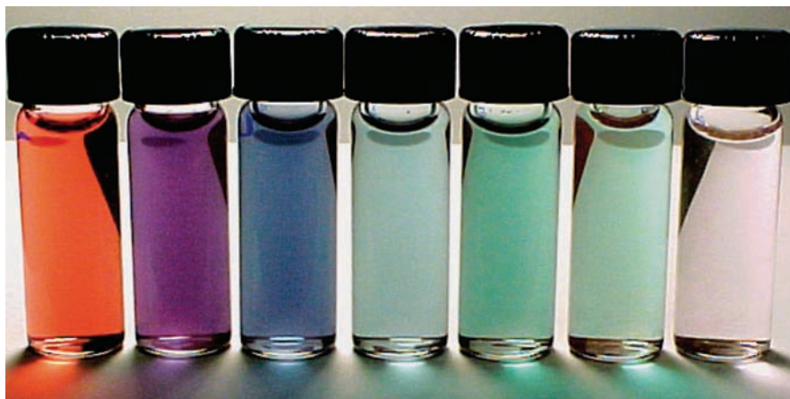
Figure 1.18 Photograph showing colors of gold nanoshell particles with different shell thicknesses dispersed in water. Core : shell ratio decreases from left to right. (Photo by C. Rodloff. Courtesy of Professor Halas's group of Rice University, USA.)
