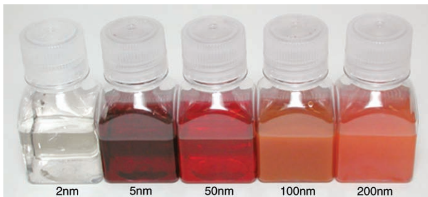
Figure 1.12 Monodispersed gold nanoparticles of different sizes (2–200 nm) in water. Note the different colors due to different light interactions, which are dominated by particle size. (Courtesy of Ted Pella, Inc., available on the World Wide Web at http://www.tedpella.com/gold_html/goldsols.htm .)
