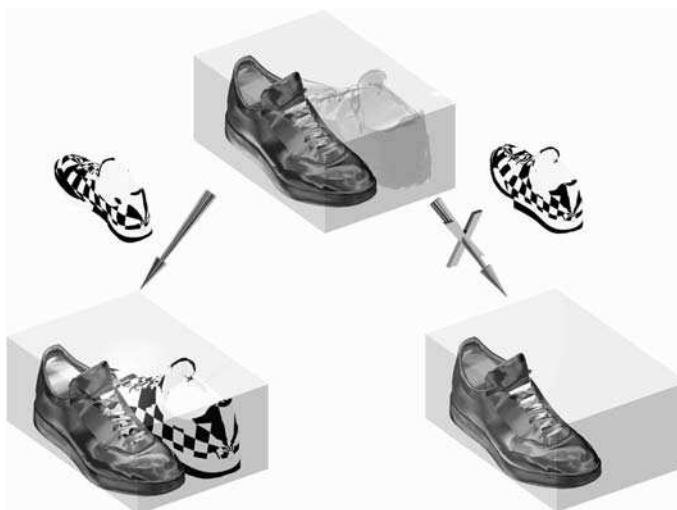
Figure 2.26 A right shoe in a shoe box leaves a chiral space that can more easily accommodate a left shoe rather than another right shoe because of the reciprocal sensing of chirality imposed by the small space available.
