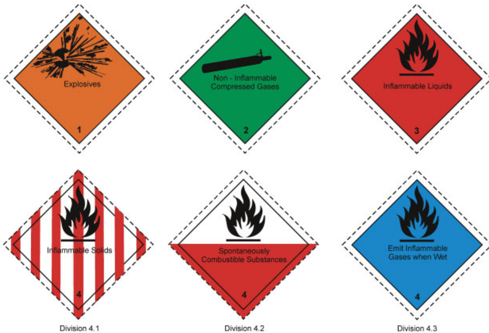
Figure 6.2 Symbols for transport of dangerous goods by road. Based on the 'Transport of Dangerous Goods (Recommendations Prepared by the United
