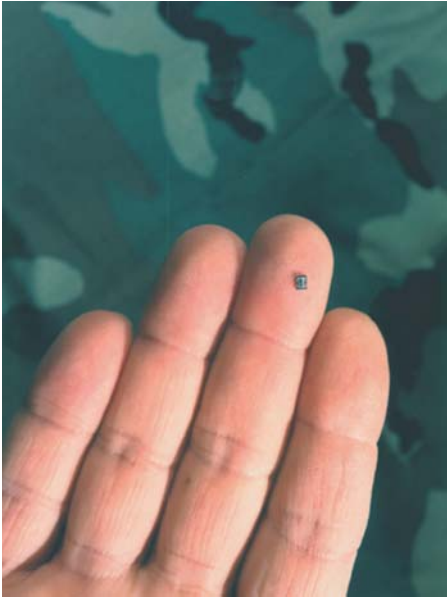
▲ Figure 1-2 Wireless body temperature sensor will communicate soldier's physical state to a medic's helmet. (Courtesy of ORNL)
