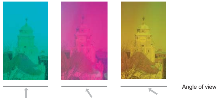
▲ Figure 6-4 Radiant mirror film. The color of the transparent film depends on the angle of the viewer with respect to the film
