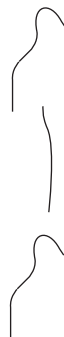
▲ Figure 4-23 In a thermally induced shape memory effect, a material can be deformed, but 'remembers' its original shape after heating. Shape memory effects may also be induced in other materials by magnetic fields
