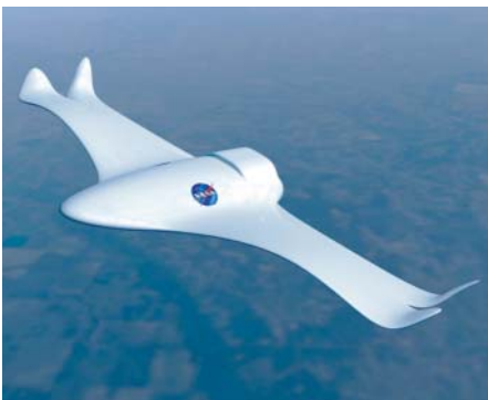
▲ Figure 1-1 NASA’s vision of a smart plane that will use smart materials to ‘morph’ in response to changing environmental conditions. (NASA LARC)
