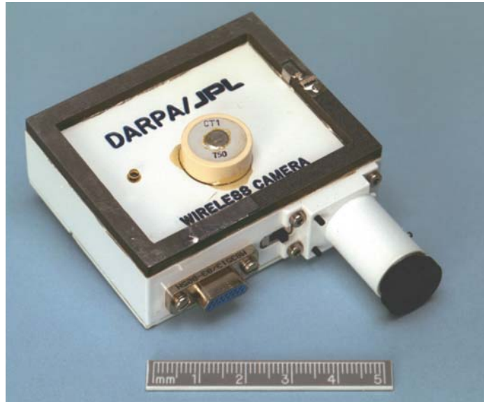
▲ Figure 5-3 The longest dimension of this experimental wireless camera is less than 10 mm. (NASA)
