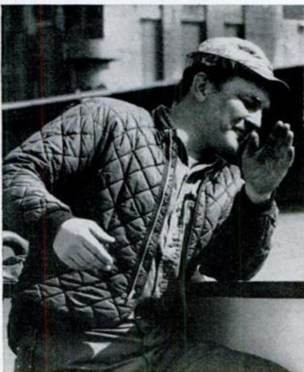
HOOK TENDER at Boeing's 747 plant gives signal to overhead crane operator to lift "micro" (slowly). Men have radios, but it's impractical to have separate frequencies for each operator, floorman
