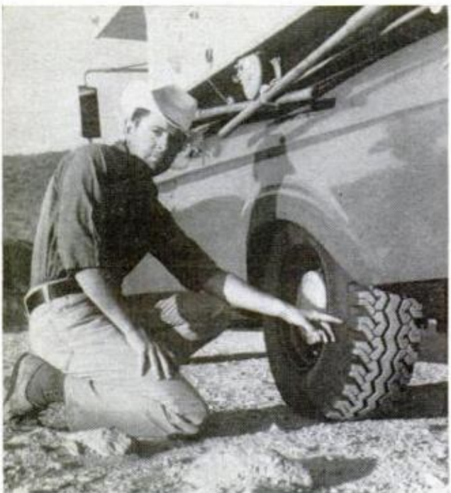
SUPERWIDE TIRES double the footprint and provide improved stability, extra flotation and more traction
