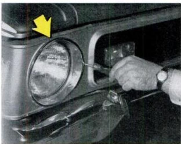
ADJUSTMENT OF HEADLIGHT in the horizontal plane on this car is made through hole near side of headlight. Vertical adjustment screw is reached through opening where top of the fender meets grille (arrow)
