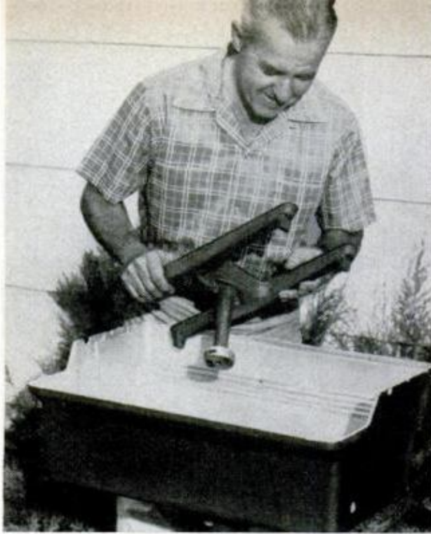
BURNER IS PLACED in bottom of pit and air mixer lowered into hole until it fits over the orifice cap
