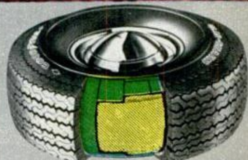
New GLAS-GUARD tire: 2 fiberglass belts and 4 nylon cord body plies for extra protection.
