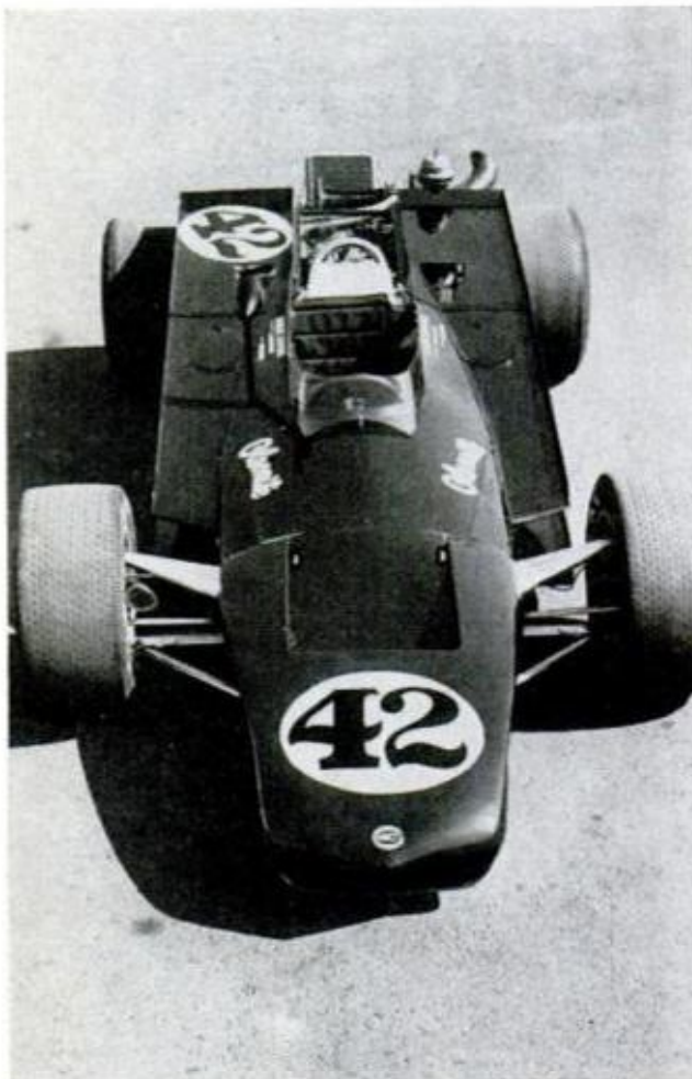
'71 EAGLE PROTOTYPE as it appeared earlier this year. Car ran in this configuration at first USAC race in Argentina where Swede Savage placed fourth. Car will be essentially same for Indy this month. It uses prominent side fins for aerodynamic downforce instead of the usual transversely mounted rear wing
