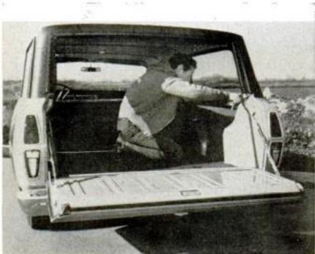
SPARE TIRE rests in compartment at right of cargo area. Both rear benches fold for a huge payload bay
