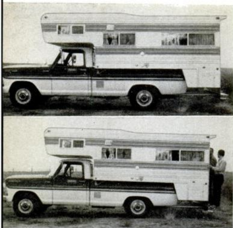
COMFORTABLY LOADED CAMPER (top) is also shown listing badly to the rear (below) because of a party inside. Overloading in this way is quite dangerous
