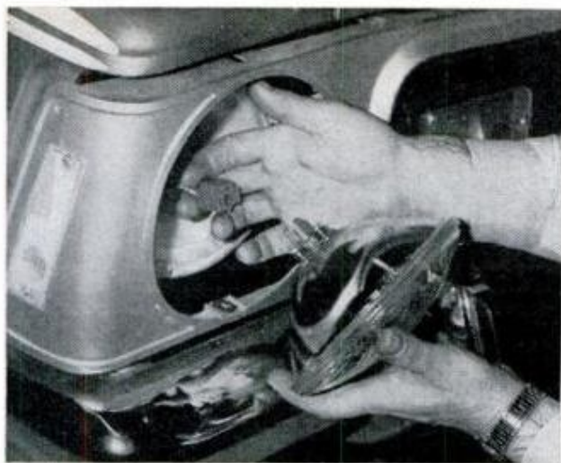
SEALED-BEAM HEADLIGHTS are very easy to replace. The three-connector plug just slides onto the prongs
