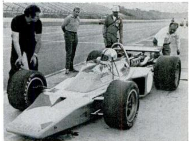
DENIS HULME , Can-Am champion, tests new McLaren M16 designed for '71 season. Note front-wheel suspension moved inside body shell to allow smooth airflow to radiators repositioned beside the driver
