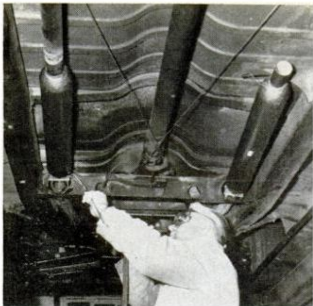
SWITCH EXHAUST PIPE from single to twin system to increase performance, reduce heat load on engine
