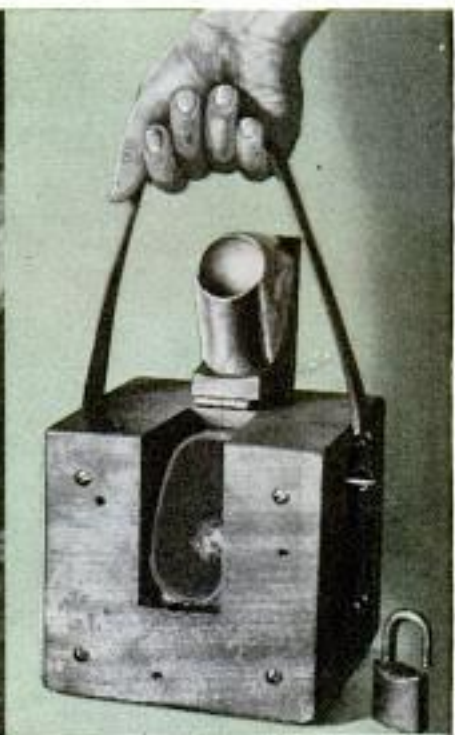
Radium sulfate is transported in lead-lined carrying case
