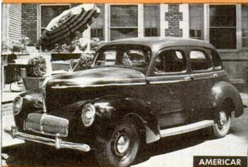
Another gas-saver is the Willys Americar, rated at close to 35 miles per gallon. It has iron alloy pistons. Enamel is used instead of chrome plating where parts are not subject to weather ravages, thus helping to conserve materials vital to national defense
