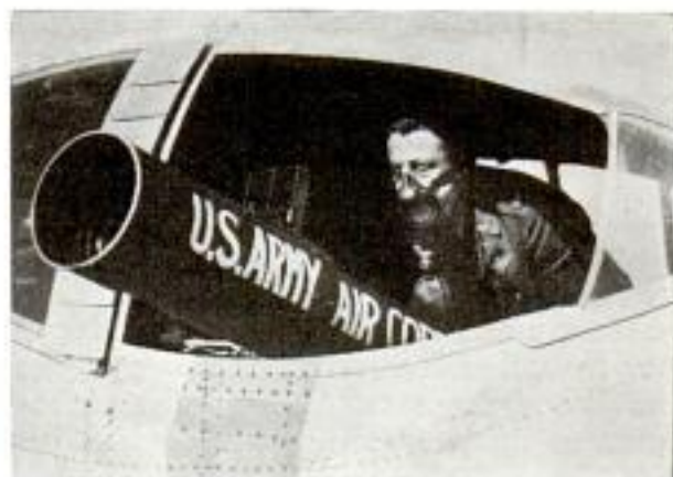
U. S. Army's giant 60-inch telephoto camera being operated by Lt. Col. Goddard
