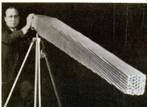
Highly directional microphone picks up distant sounds
