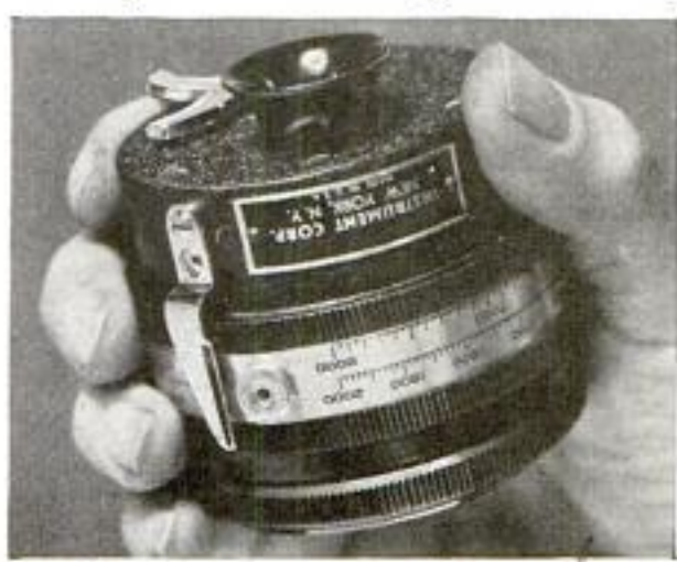
Sighting through the eyepiece, operator turns the housing until the engine or machine appears to be standing still, then reads dial
