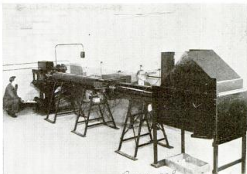
Machine automatically tees up golf ball and drives it through 15-foot tube, recording its speed, distance ability and other qualities
