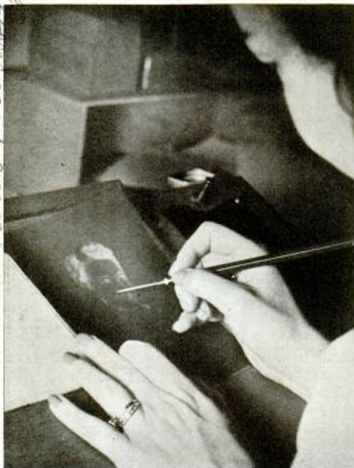
Softening a line on the negative by filling in with pencil. Notice the extremely sharp point of the retouching pencil
