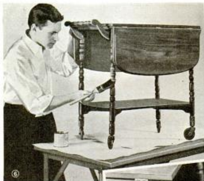
Apply a coat of raw linseed oil and turpentine to the sanded work, wipe off after 30 min., and then let the work stand overnight
