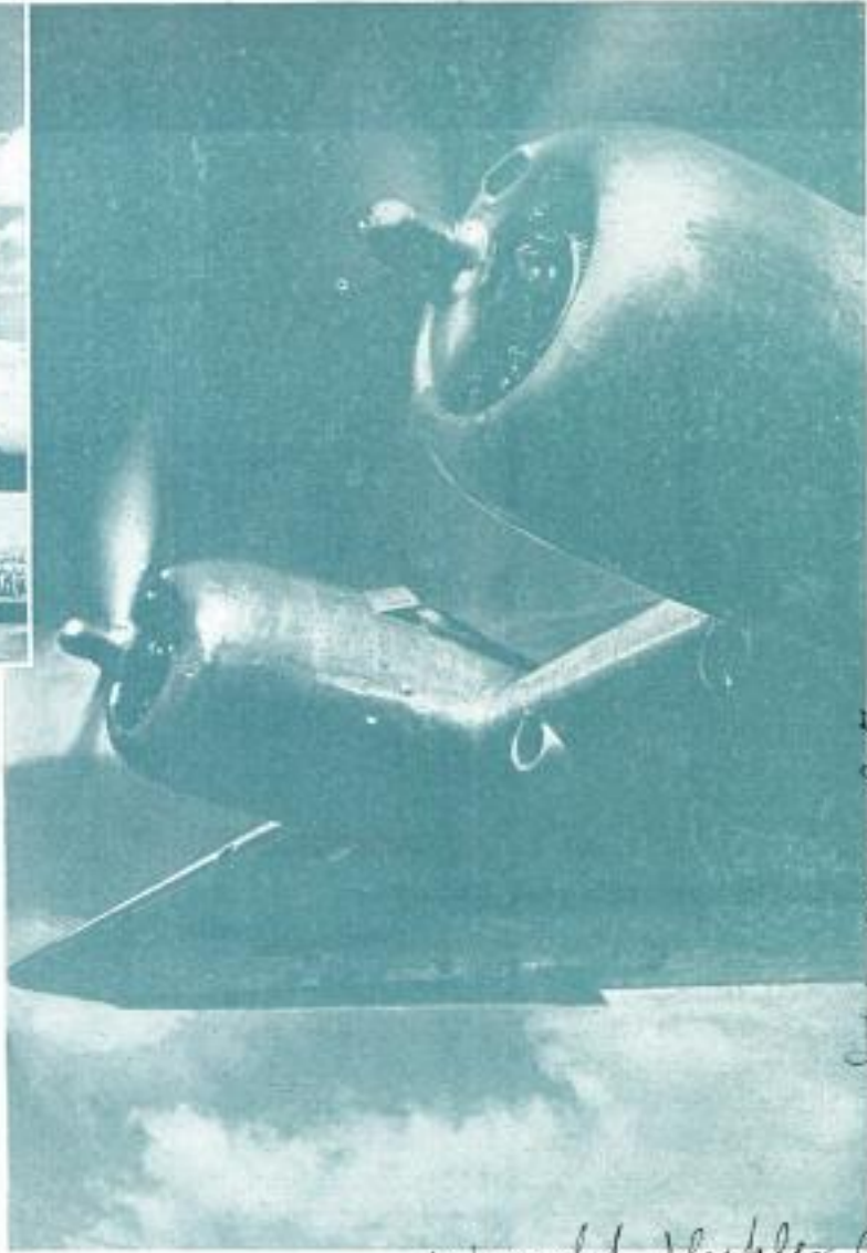
The air throbs with the beat of four 2,000-horsepower engines. Here the propellers of two right wing motors flash in the sun
