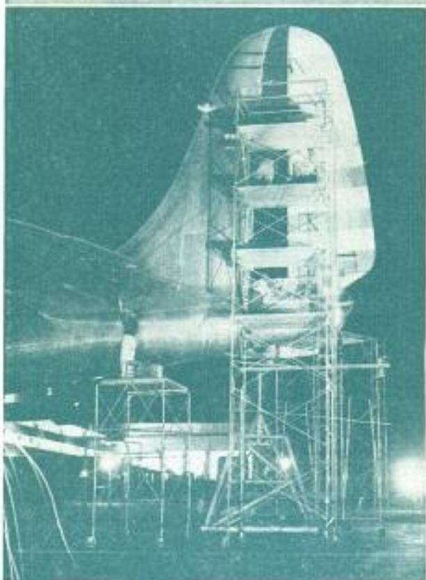
↑ Test engineers on skyscraper scaffolds are running vibration tests on tail group flaps
