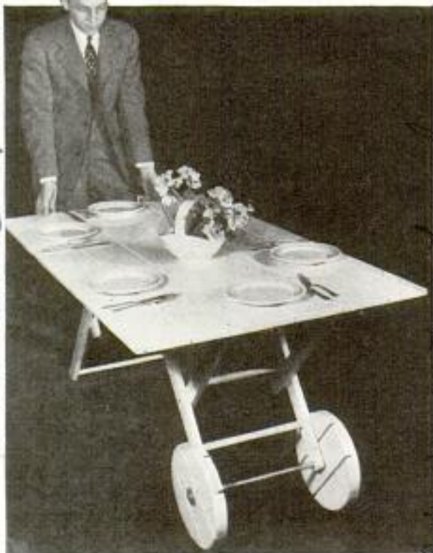
Two wheels at one end make lawn table easy to move like a wheelbarrow to a shady or more pleasant spot
