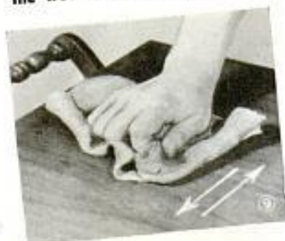
Follow the oil treatment with a coat of boiled oil and drier and let dry until tacky; then rub it off across the wood grain
