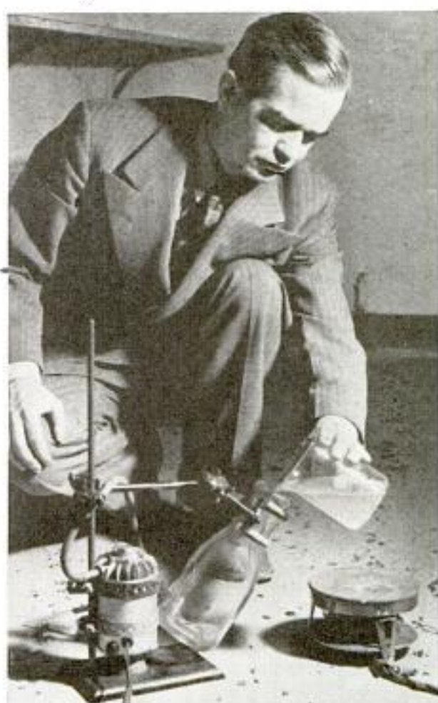
Insecticide is vaporized when sprayed on hot plate
