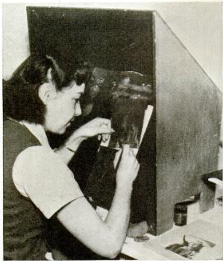
Working in a special booth that has side and front walls, the retoucher is free from extraneous light and reflections
