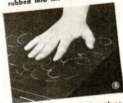
After 12 hrs., apply from three to six coats of boiled oil 24 hrs. apart, rubbing each coat into the wood with the bare hands
