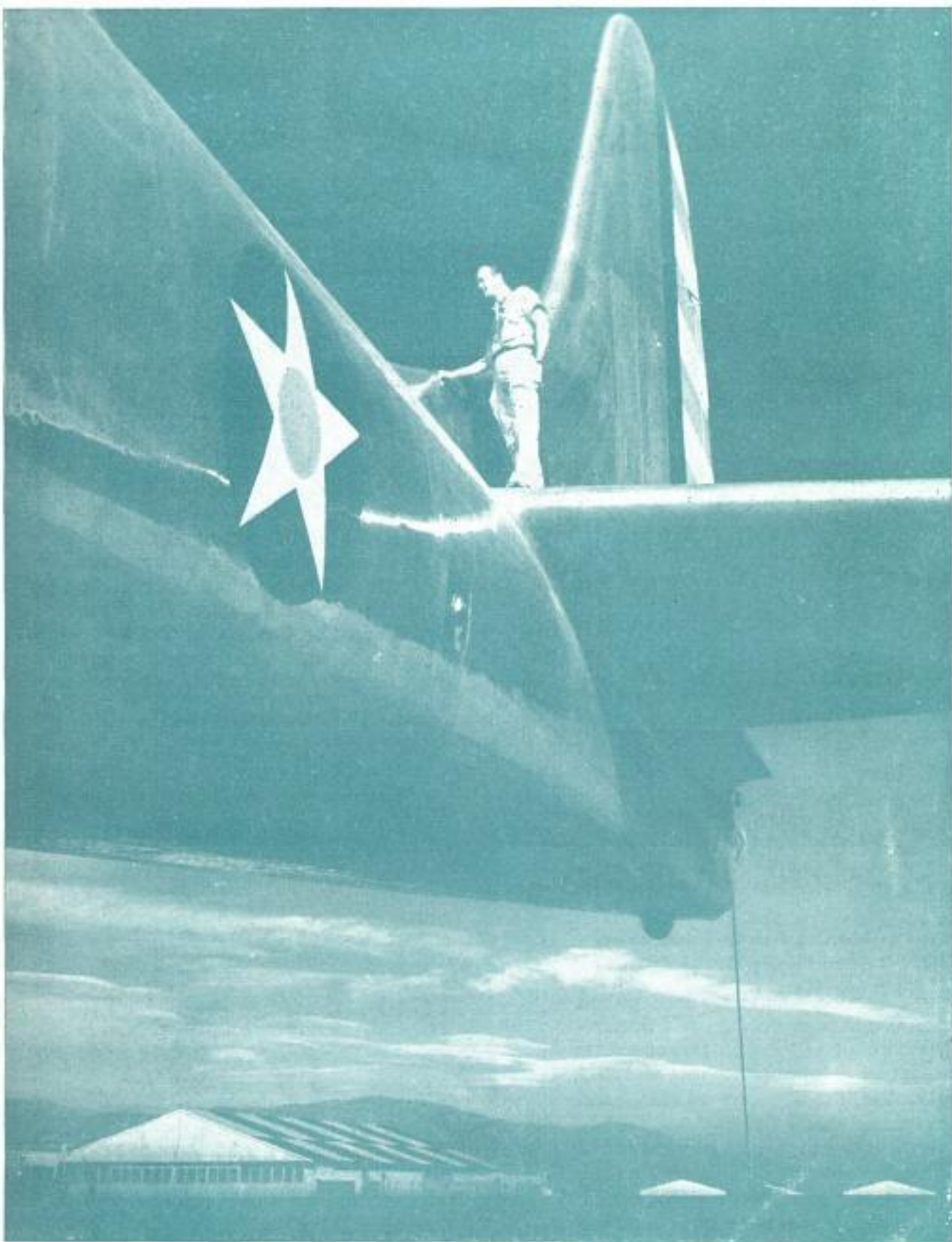
Inspecting the "skyscraping" tail surfaces of the B-19. The rudder alone has 237 square feet of movable surface. Huge as it is, Colonel Umstead believes it is but the forerunner of far larger planes of 500-passenger capacity, or greater, which will be built when there is a need for them
