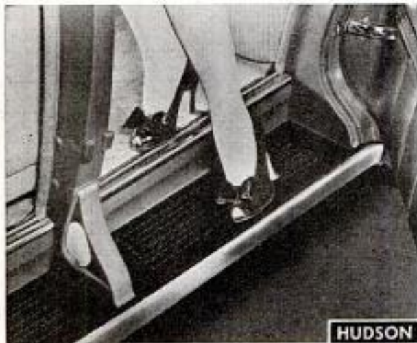
Wide, full-length running boards, concealed by the bottom of doors, are used by Hudson
