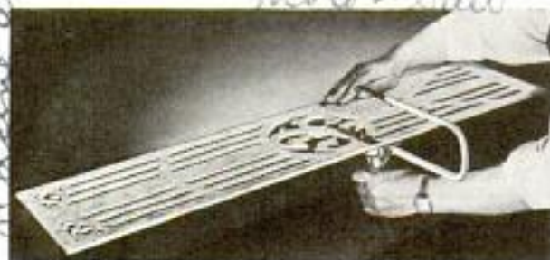
Long cuts in panel were made with blade set sidewise
