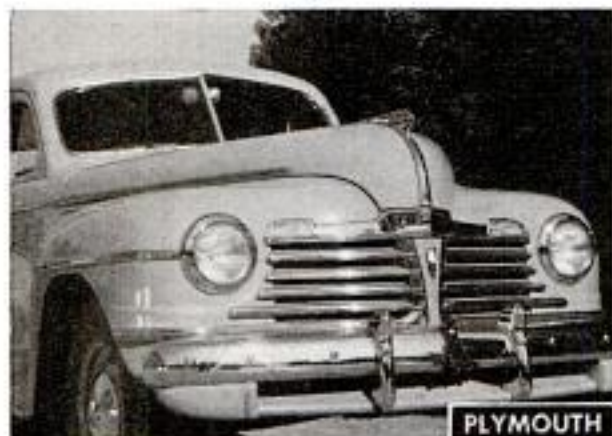
Below the Plymouth bumper is an air scoop that makes the cooling system more efficient
