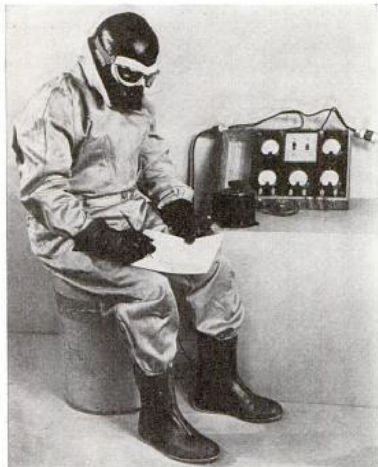
Here is one of the electrically heated flying suits, designed for the U. S. Army Air Forces, undergoing test in a cold room
