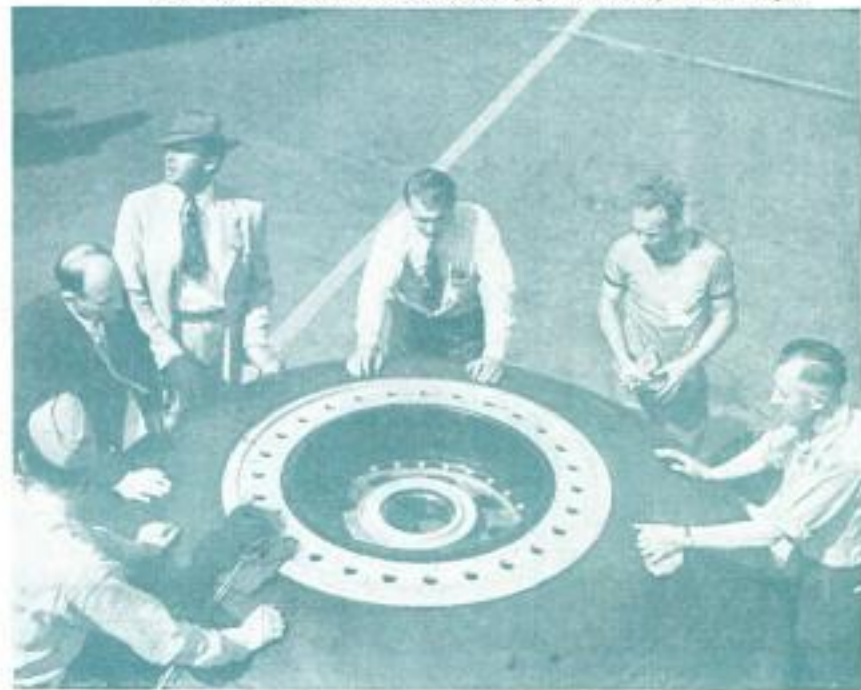
Engineers gather around one of the giant wheels to inspect it after exhaustive brake tests. The 24-ply tire is eight feet high
