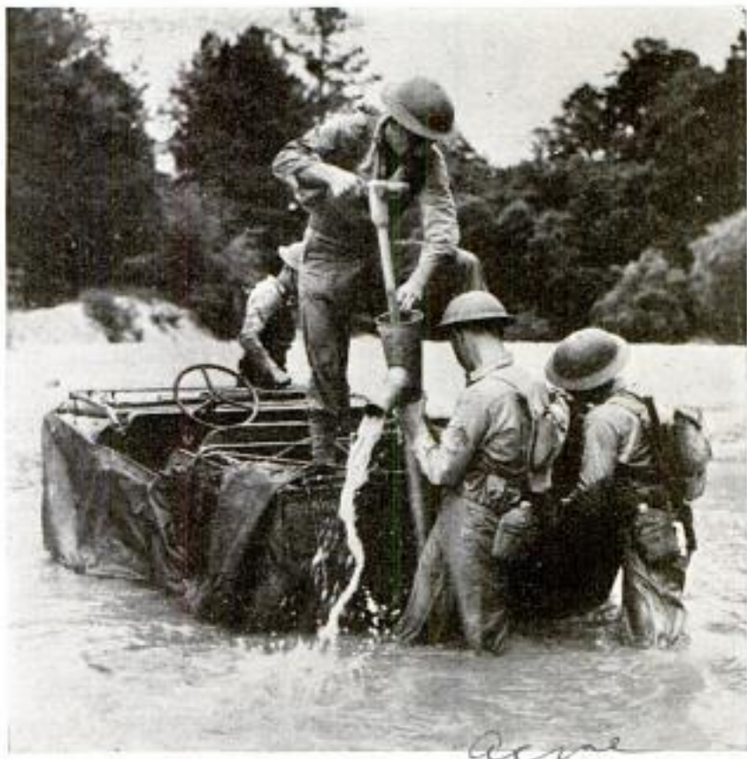
Soldiers wrap scout car in canvas, then pump out water to make it float
