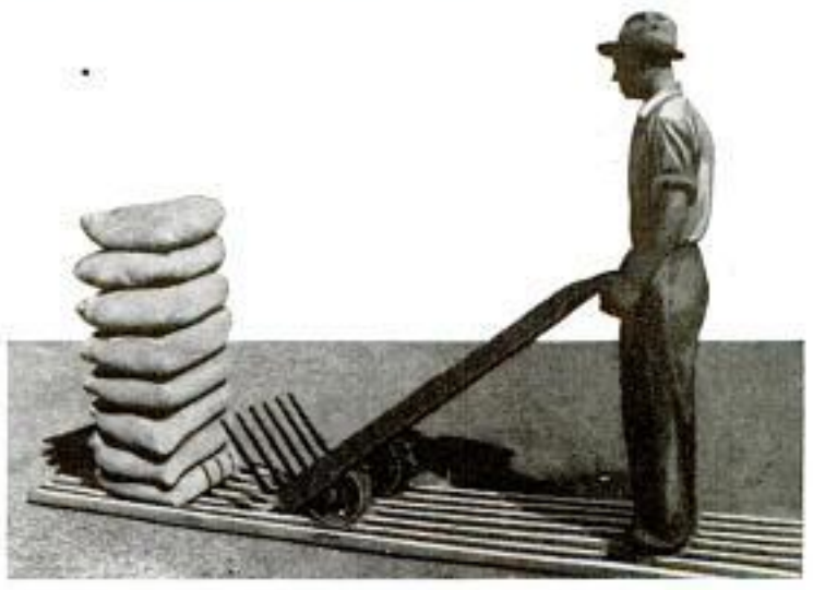
Steel fingers slide in spaces between boards to pick up load
