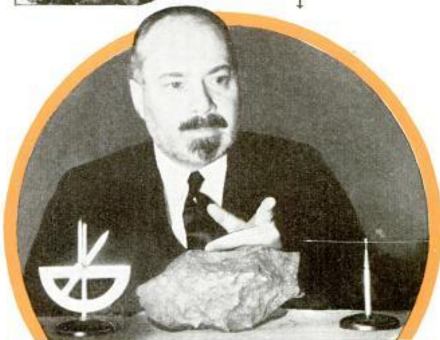
Determining the magnetic properties of a siderite by means of dip needles
