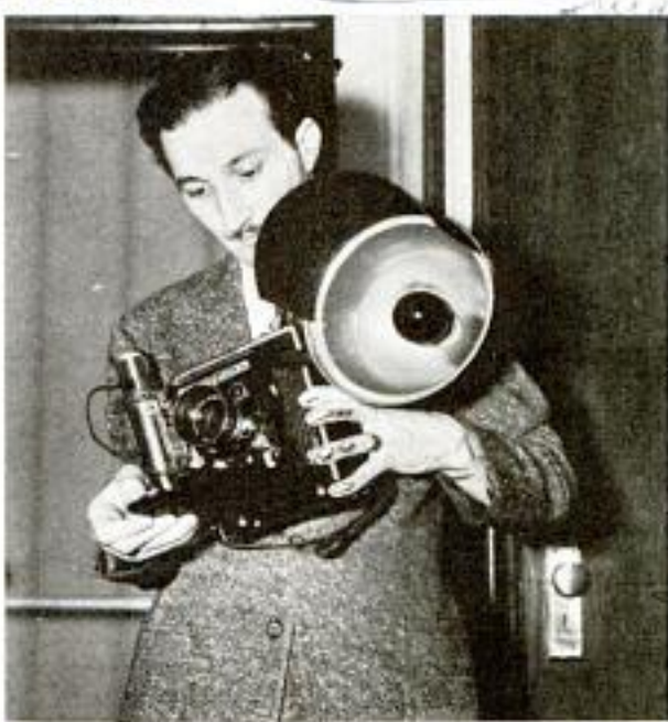
Black bulb in reflector emits only infrared light
