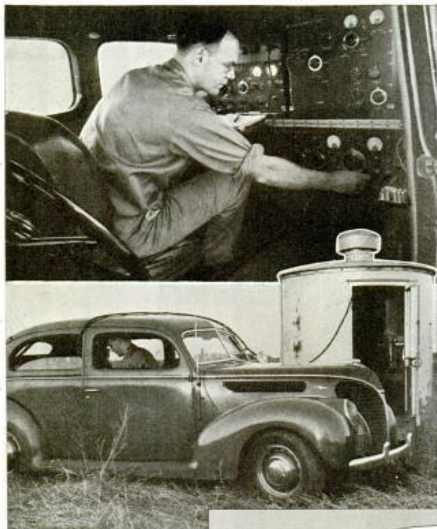
Test board of the mobile laboratory is shown at top; it occupies rear seat section of sedan. In the center is the car during a test of coaxial cable, and at right a diagram of its equipment
