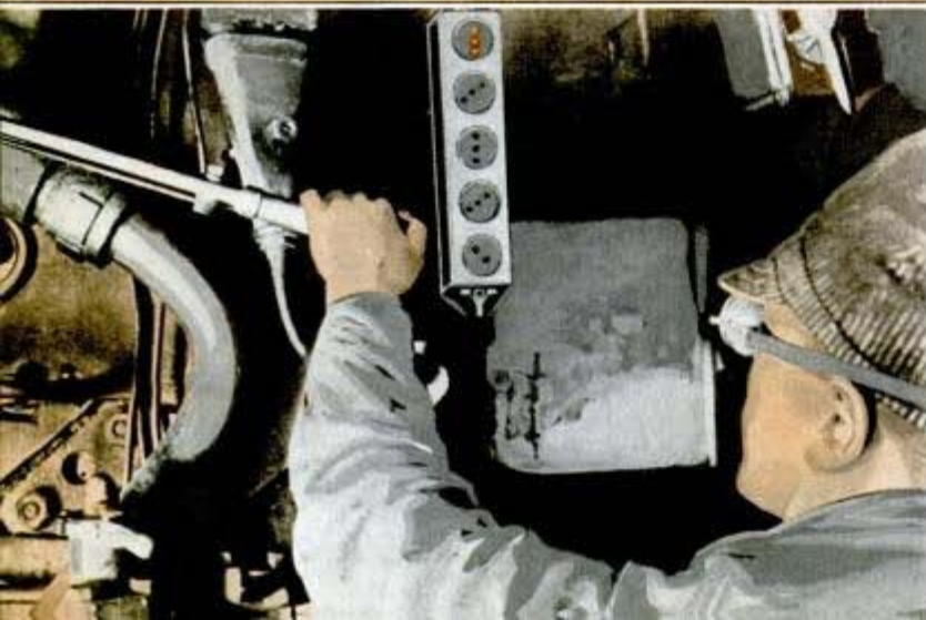
Block signals are brought right into the cab of modern locomotives. Left, a Pennsylvania engineer watches panel which reproduces track signals
