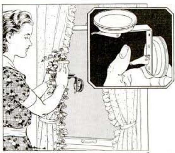
One suction cup grips window, other holds article
