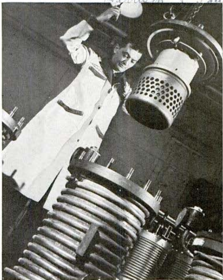
Assembling an ignitron at Westinghouse plant, East Pittsburgh. It is used to change alternating into direct current for aluminum manufacture
