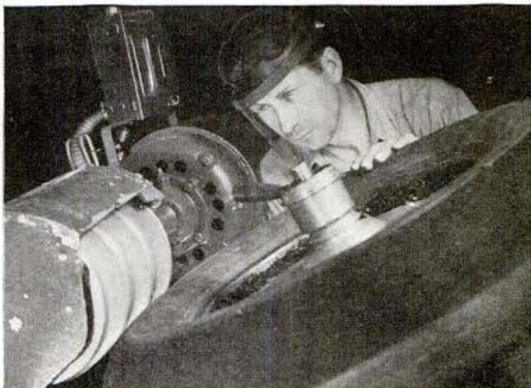
↑ Buffing a tire in Goodyear recapping station. Note mask that protects operator's face. Recapping costs about one-third the price of new tire
