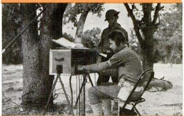
Portable field telephone exchange set up near mobile headquarters
