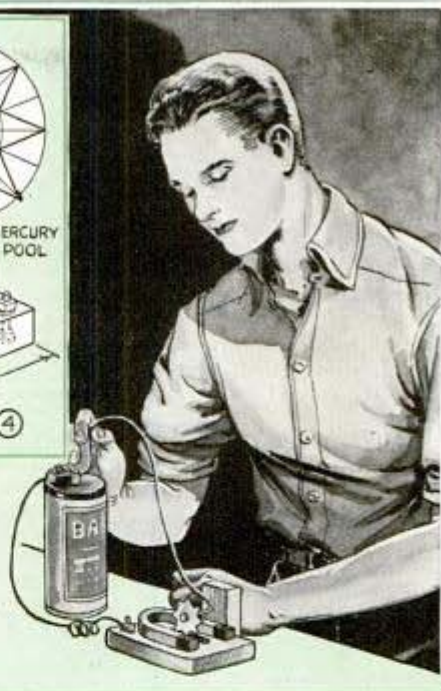
Barlow's wheel: An 8-pointed star of thin brass or aluminum, which rotates when the tips contact mercury in pool at base and direct current is applied
