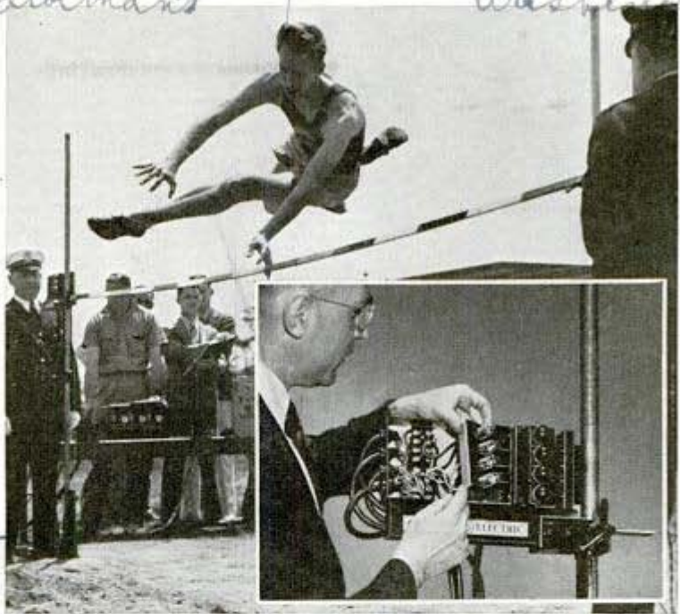
High jumper clears the bar with inches to spare, and battery of electric eyes on post gives him credit. Lower view shows assembly of photocells
