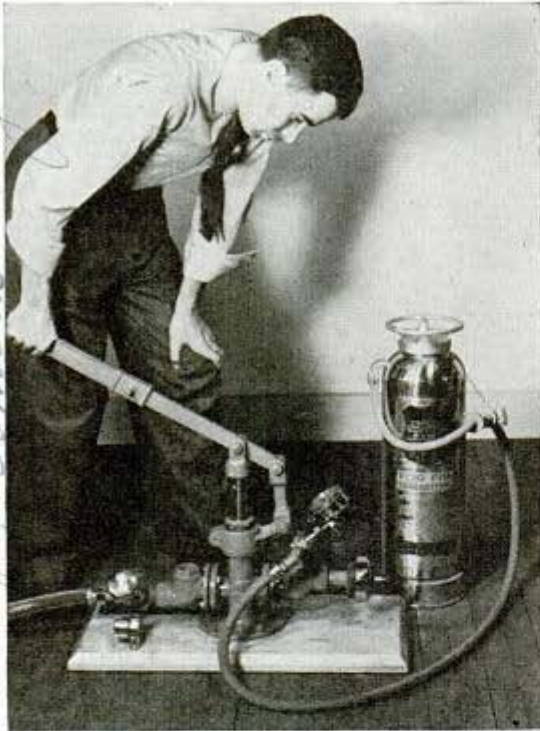
Portable pump creates pressure to test extinguisher
