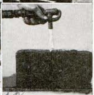
Thirty-minute water test does not affect adobe-and-asphalt brick above, but untreated mud brick below crumbles
