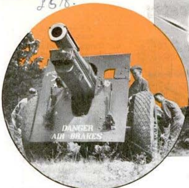
↑ View of 155-millimeter gun, motor-driven unit which can hurl a 95-pound projectile ten miles or more in defense of our shores
