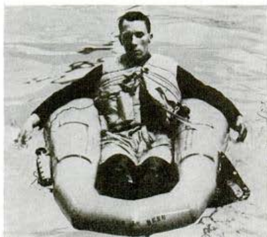
Compressed air from bottle at left inflates lifeboat
