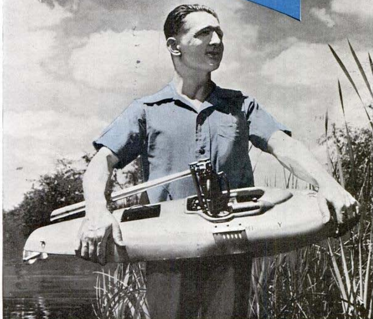
Wolfgang Pfister holding class A hydroplane powered by air-cooled gas engine with overhead valves. Note long exhaust pipe. The craft has made 40 miles per hour. Hull is carved balsa wood covered with cloth.
