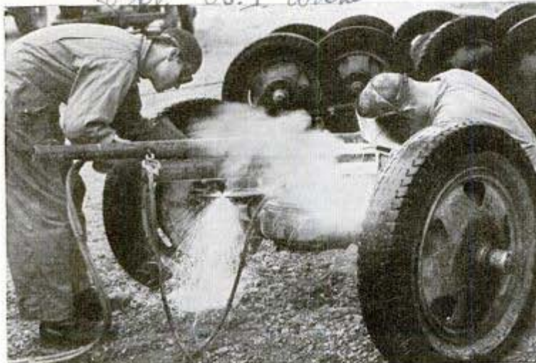
Ordnance men assembling dummy gun with acetylene and electric welders
