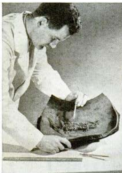
Inspecting inside of a tire section to determine cause of failure
