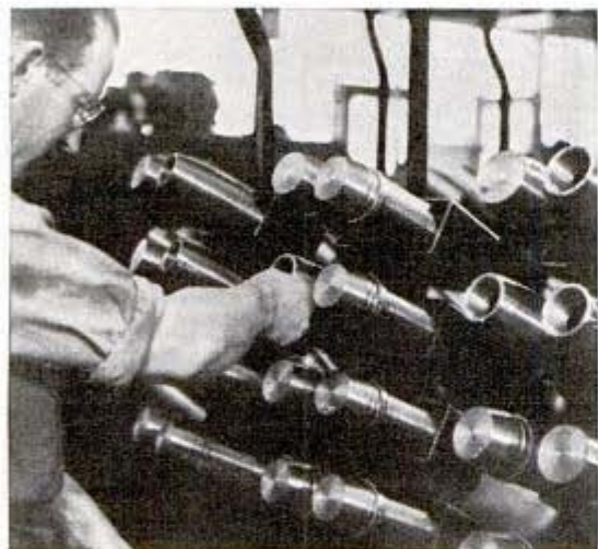
Inspecting nose diameter of 75-mm. shells produced in volume with machine tools
