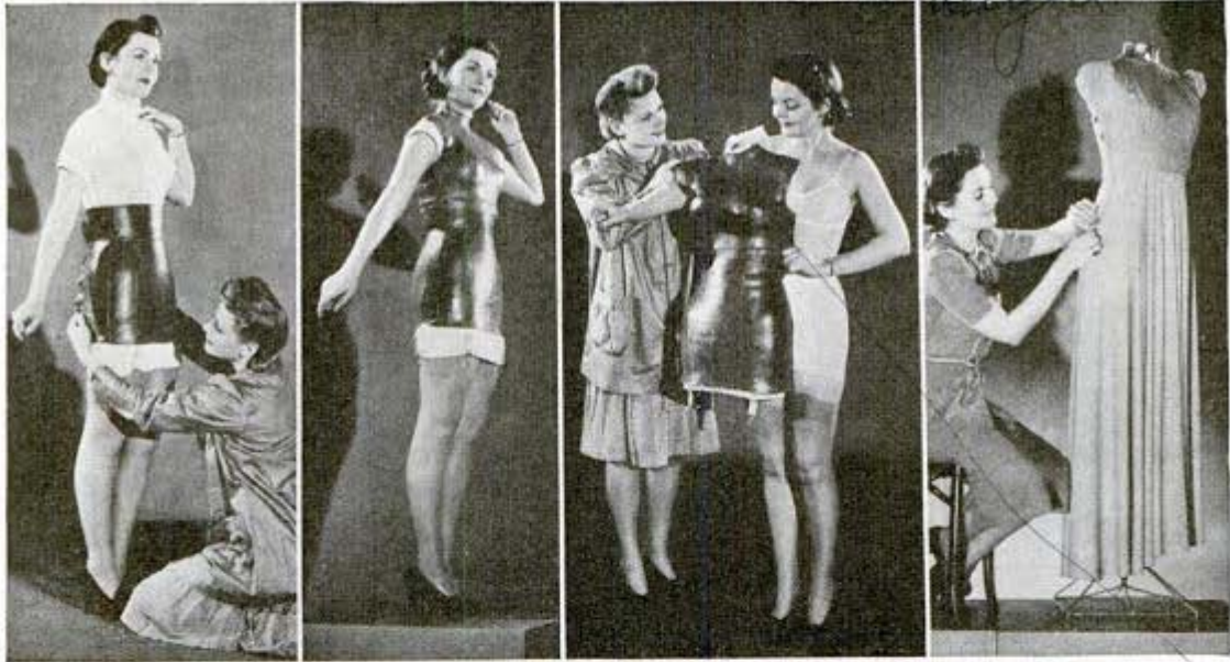
Left to right shows steps in molding plastics to figure, and how garment is fitted to dress form
