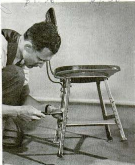
To raise chair, the lower end of each leg is unfastened, extended and bolted in new place
