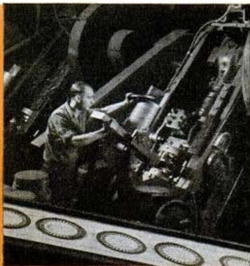
Huge press punches out stator laminations used in electric motors
