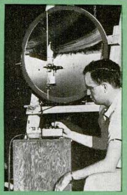
↑ Apparatus comprising “infrared telescope” used for measuring so-called black body radiation of atmosphere
