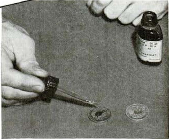
Below, testing real and spurious coins with acid, a quick and simple method
