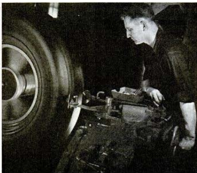
Stitching tread on a tire being recapped—one of the last steps in the operation. Many stations are ready to do this job for motorists
