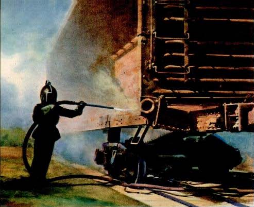
Sandblaster at left wears "diving" helmet and breathes through charcoal filters while directing air and sand blast against steel boxcar, whisking off rust and dirt so car can be repainted
