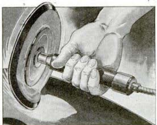
Note how sanding disk flexes to fit curved surface
