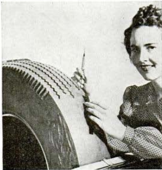
Expert modeler carves a new tire design in clay
