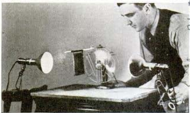
Negative drying between two infrared lamps with aid of fan
