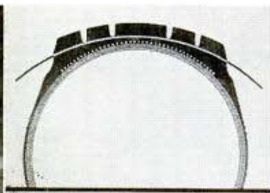
Drawing shows how much rubber is left on tire after tread wears off
