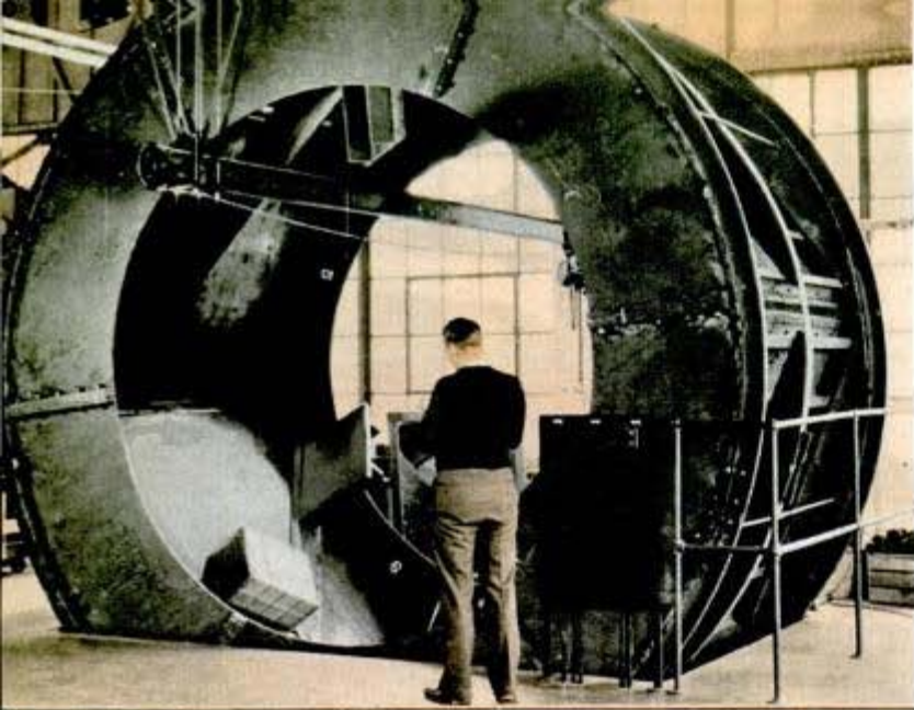
Better ways of packing and loading freight are one subject of railway research. Above, a container-testing machine gives a carton a rough ride
