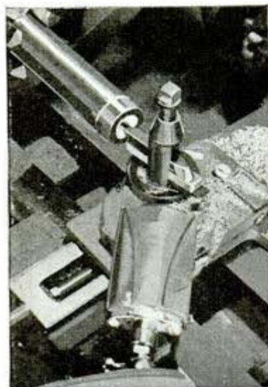
In order to get tight-fitting parts that screw together, a number of special cutting tools like the ones shown below are made up and very light cuts are taken
