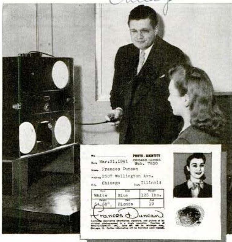
Camera makes photographic identification card, like sample, including descriptive details, fingerprint, and a picture of the subject
