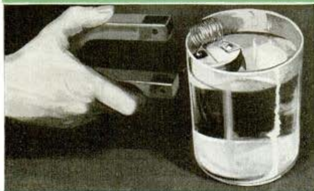
De la Rive's float: Coil on block floats in acidulated water. Slight current is generated and a magnetic field is produced, making coil susceptible to influence of a permanent magnet
