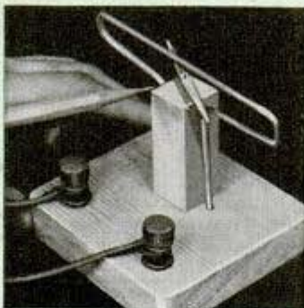
Perfectly balanced on a phonograph needle, a magnetized needle of sheet iron will respond, the extent of movement varying with current applied through coil surrounding it
