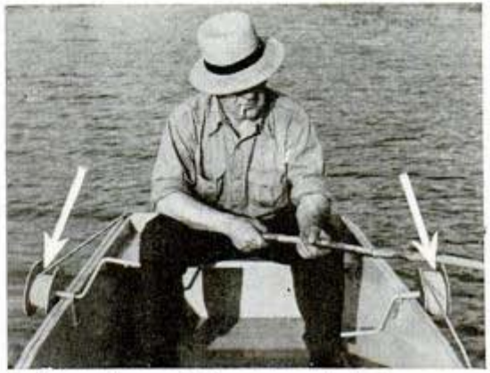
Anchor reels are within easy reach of the oarsman so he can raise the anchor without leaving his seat
