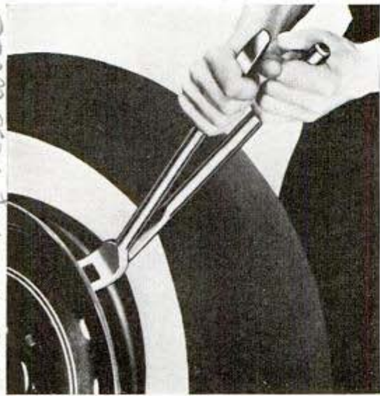
Twin-handled prying tool supplies powerful leverage to remove tires from wheels without using hammer
