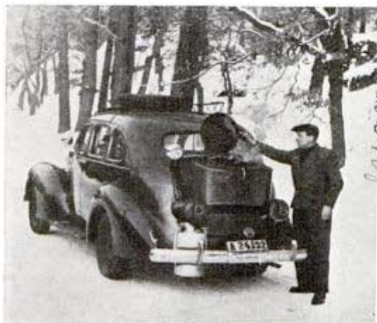
Charcoal burner on rear drove this car to victory
