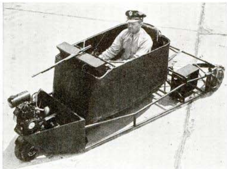
Cockpit of the "pilot buggy" banks and tilts in response to standard airplane controls, giving the pilot effective "flight" training on the ground
