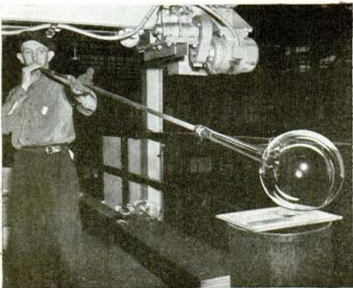
Workman blowing test flask taken from 900-ton furnace for analysis
