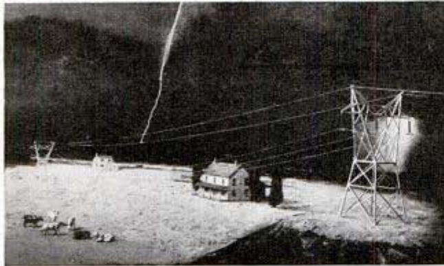
Two research engineers inspecting miniature power line to determine effects of man-made lightning upon cables protected by two "lightning rods" strung above them
