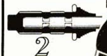
2 Bosses are swaged into blade recesses. Four sharp wings are swaged on outside of bolster. Blade is now locked into bolster . . .
