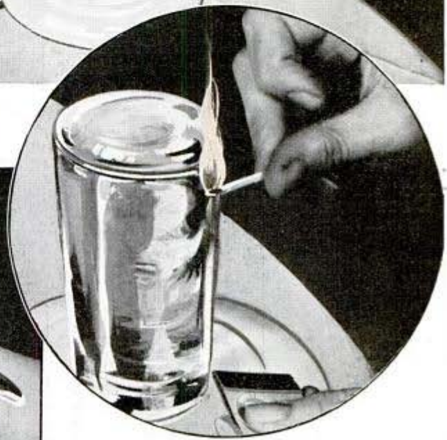
The glass is filled to overflowing or to the point where, due to surface tension, water rises above lip of glass. Heat applied near lip makes it overflow.
