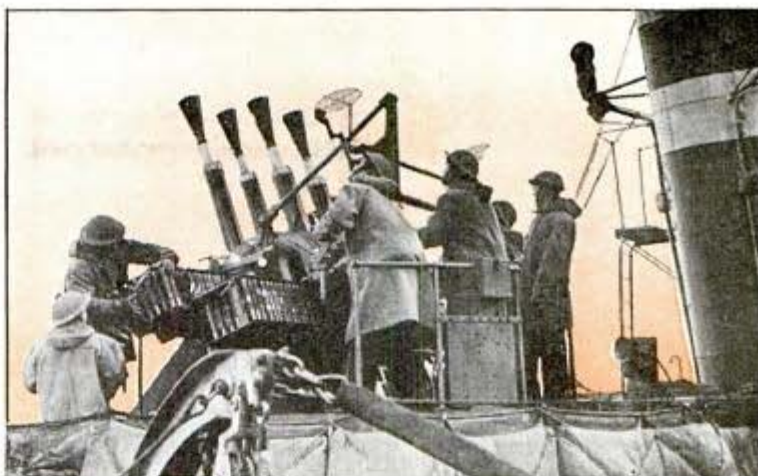
Feeding shells into the "pom poms" of a Polish destroyer with the British fleet. These multiple rapid-fire guns can fling a tremendous weight of metal into the sky to drive off enemy bombing planes
