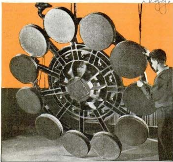
Big polishers, like the one shown above, are used to put a high polish on safety plate glass produced for automobiles at the Ford factory
