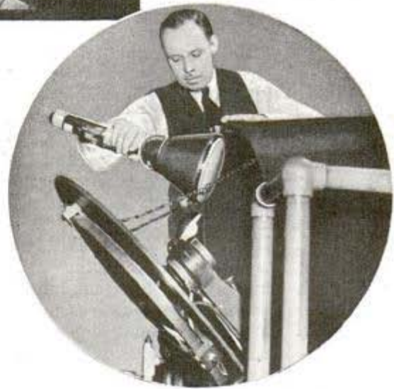
Inserting the kinescope, the large television tube on which picture is formed, into projector
