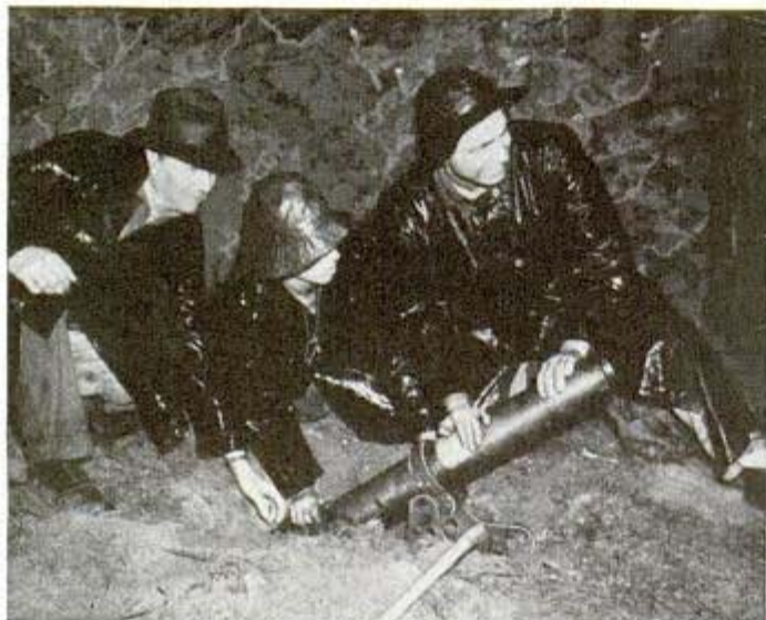
Cannon below fired a line across 600 feet of water to establish communication between banks
