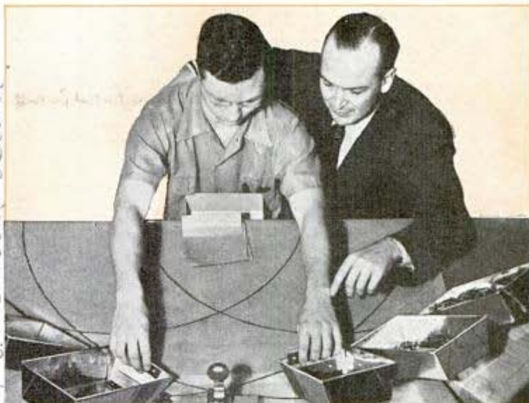
California Institute of Technology films time-motion study; arcs on table show worker where he should use each hand. Below, war canoes in tank for miniature shot; wires will be invisible in after-dark scene
