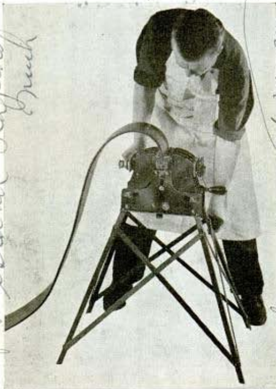
Belt lacer on stand of convenient height is light enough to be carried to the job by one man
