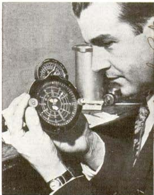
This device plots a plane's position in 15 seconds
