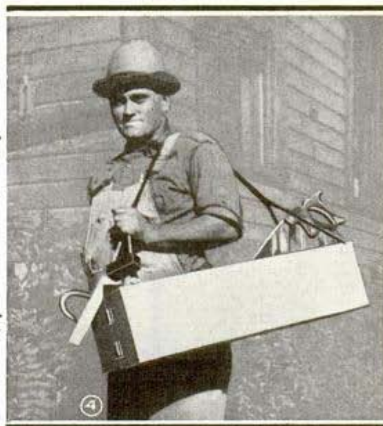
Provided with a strap or rope so that it can be slung from the shoulder when carried, this box folds flat as in Fig. 5, for convenient storage
