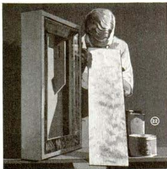
A clean board with a coat of high-gloss varnish is used for testing dry-dull varnish for brush marks. If marks show after 10 min., thin the varnish with a little turpentine
