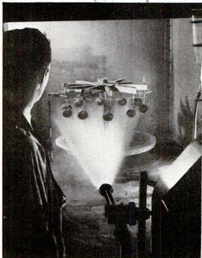
Flies buzz busily in the lethal chamber above until a scientist comes along with an air gun and shoots insecticides through the ports. Later the results are evaluated
