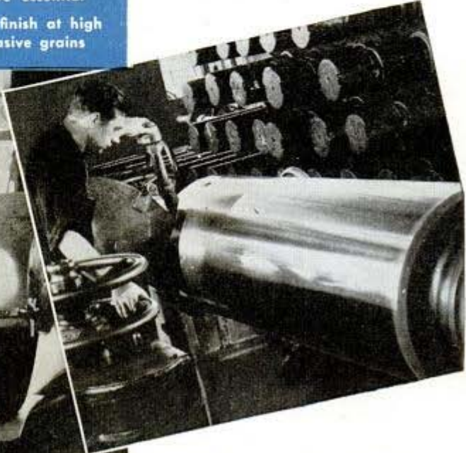
Rolls, such as are used in rolling mills (above) must be ground to exceedingly accurate dimensions and with a surface as nearly perfect as possible to insure uniform thickness of rolled sheets
