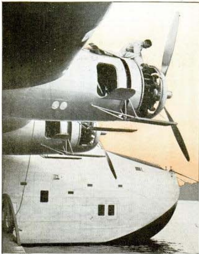
So big is the Boeing 314 Clipper that each of its four Wright Cyclone engines has its own room, accessible during a flight
