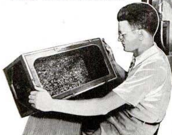
Carbon-arc lamp in greenhouse of pest-control laboratory is science's nearest approach to sun
