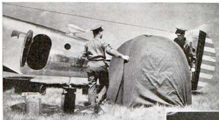
Ribs inflated with carbon dioxide support the aerial cameraman's darkroom tent
