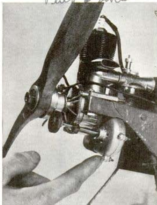
More power to the midget engine is given by installing this supercharger to produce a better gas mixture
