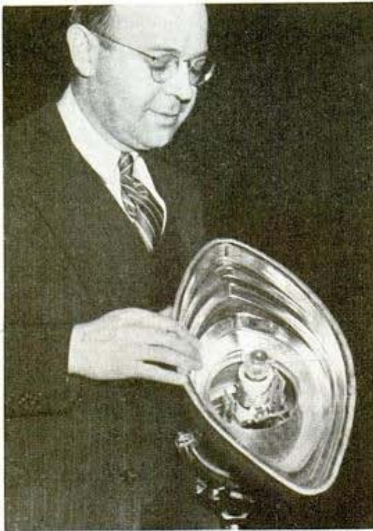
Invisible rays from this lamp make road signs readable at night. Reflector points visible rays downward
