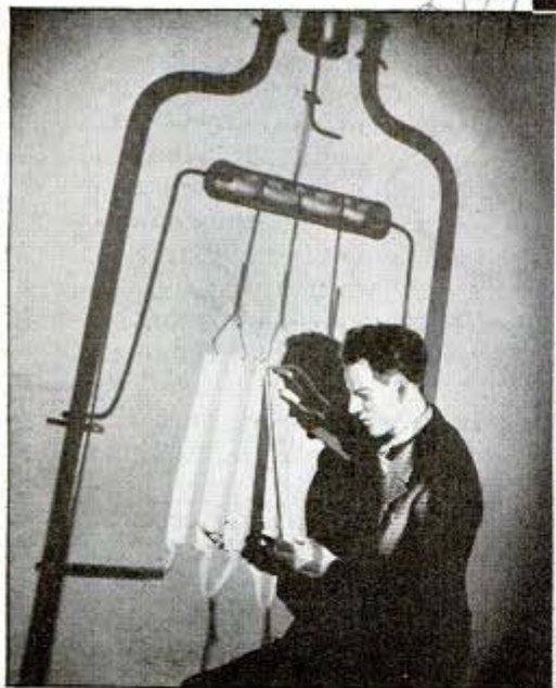
Engineer studying expansion of coils in 1,000-watt lamp by inspection of greatly enlarged image of lighted filament projected on wall
