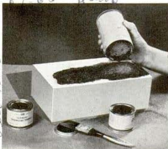
Sifting flock onto surface that has been painted with undercoat. This puts coat of felt on surface
