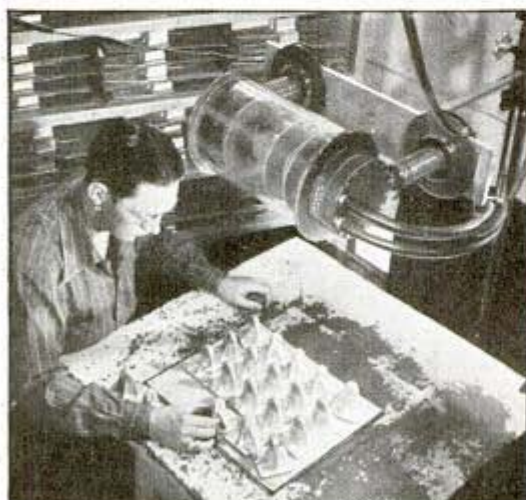
Hidden flaws in metal which might result in failure at a critical point are discovered by the X-ray. At left, an engineer prepares metal parts for the X-ray inspection; at right, examining an X-ray plate
