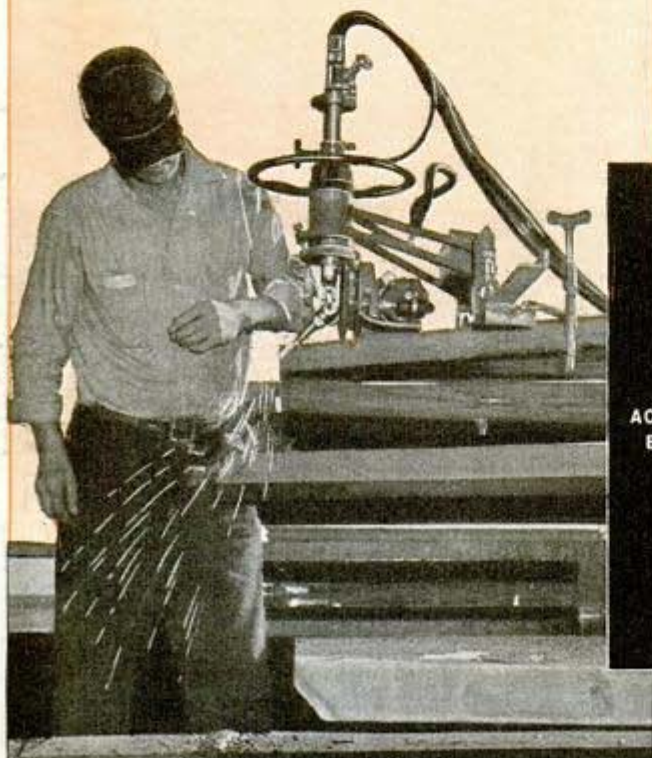
Beveling two-inch steel plates with oxy-acetylene cutting machine to fit them snugly in magnet of super-cyclotron
