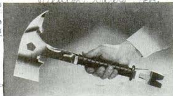
Combining several tools in one, this hatchet is efficient for rescue work in case of highway accident
