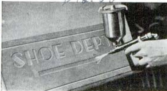
Above the sand-blast gun, which is handled like a pistol, is a half-pint cup feeding sand to the nozzle
