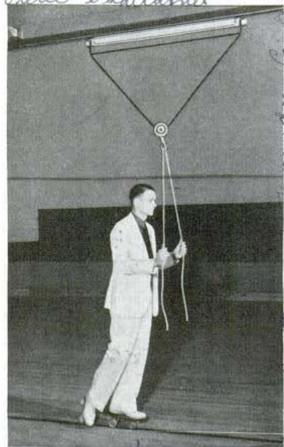
Installed on a straight or circular track at skating rink, this trolley gives the beginner confidence
