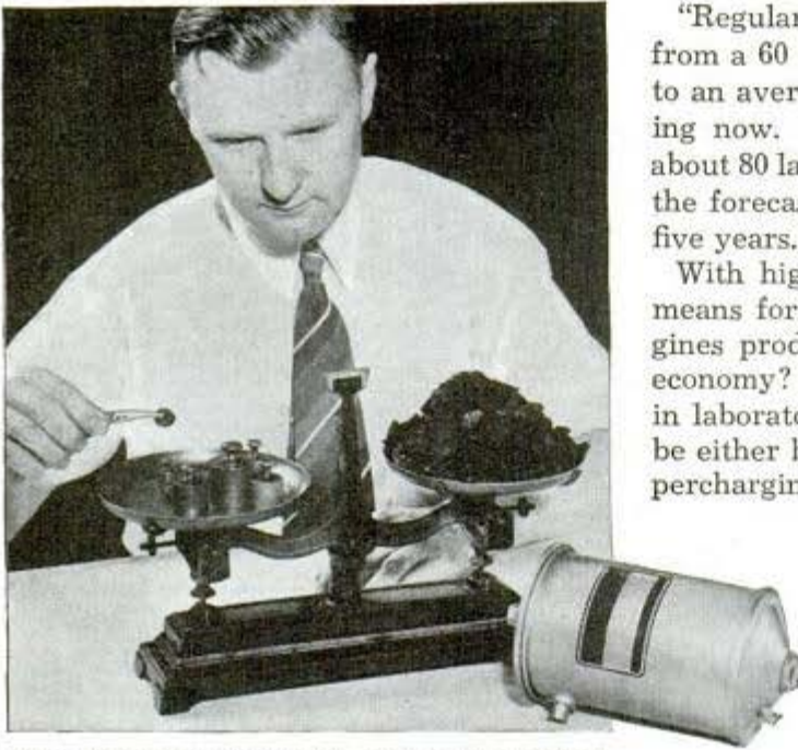
If your engine is not efficient, perhaps it is clogged. Note foreign matter, weighing one and one-quarter pounds, removed from oil by filter in 8,000 miles
