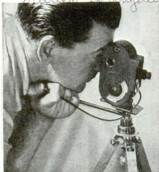
Cable release adapted to movie camera can be locked in action, allowing photographer to appear in scene
