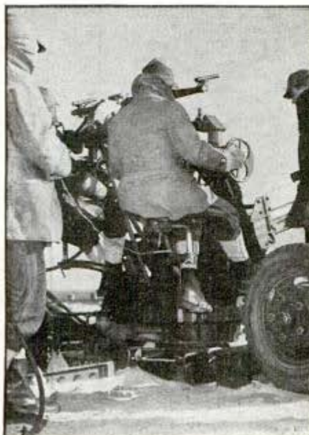
In the din of action the crew might miss "cease firing" command. Below, rope is tied to trigger foot of man firing; man behind him, alert for signals, yanks the rope at "cease fire"
