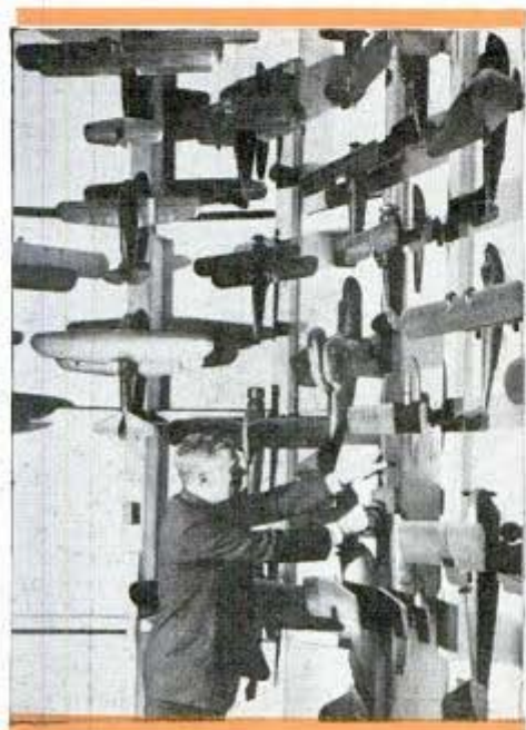
Right, model hulls are made of sugar pine, glued and doweled. In shaping and smoothing the hull, accuracy to 1/100 inch is required
