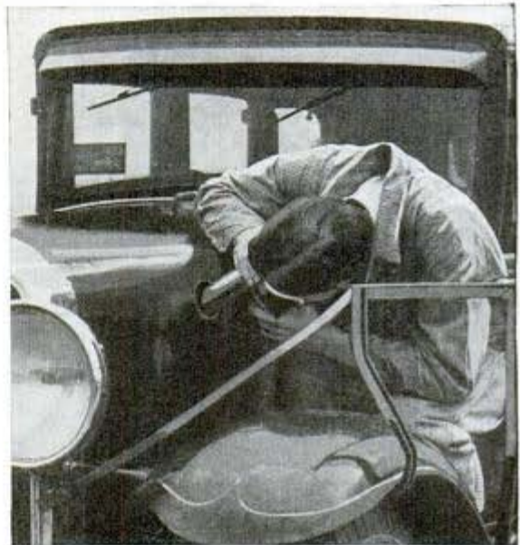
Taking reading with optical pyrometer during road test
