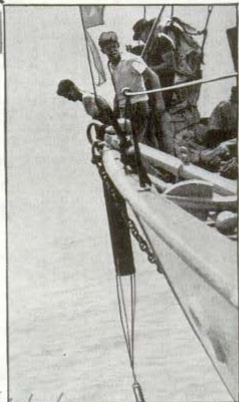
Above, diagram showing how ocean floor is mapped. Below, bomb-exploding device with float going over the side of research vessel
