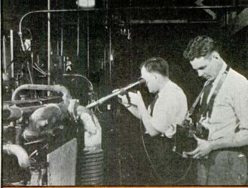
Above, research workers measuring temperature of exhaust valves. Man on left is using optical pyrometer and looking through quartz window of exhaust manifold. Below, second tractor tests first by creating resistance
