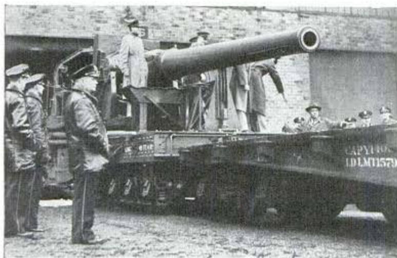
Army officers making preparations for test run of eight-inch railway gun
