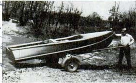
Top, winch permits man to load boat on trailer unassisted; bottom, launching boat in water is also easy
