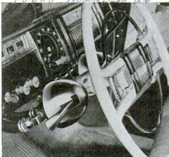
Bell-shaped housings beneath steering wheel contain levers to operate clutch and brakes by vacuum power
