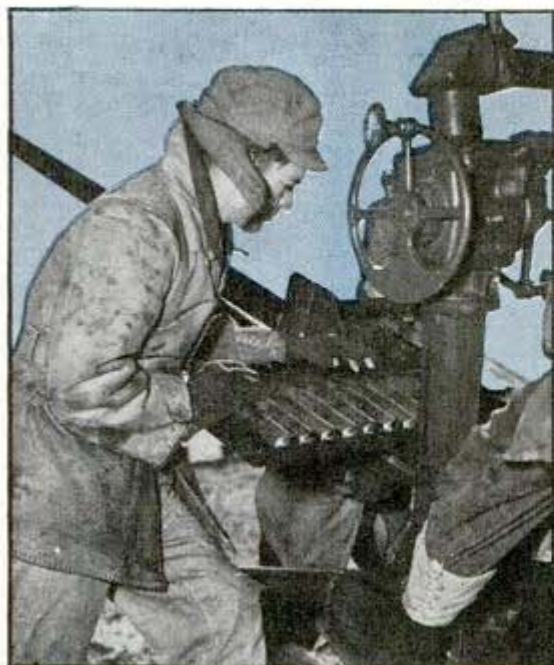
The loader (above) is kept hopping to feed clips of ammunition into the anti-aircraft gun. Its rate of fire is 120 rounds per minute
