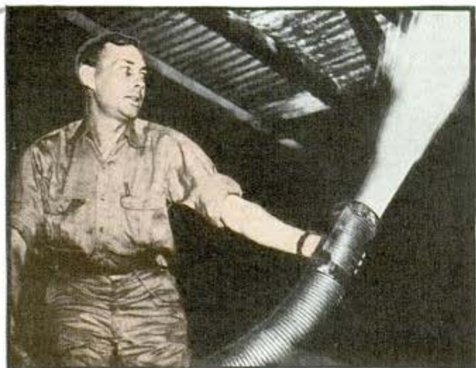
Controlling a writhing snow gun, which fires 10 to 15 tons of snow an hour, is not easy
