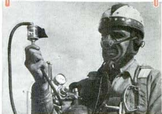
Pilot ready, with oxygen tube hooked up to supply in plane. Below, dancing pith balls in small cage show if oxygen is flowing
