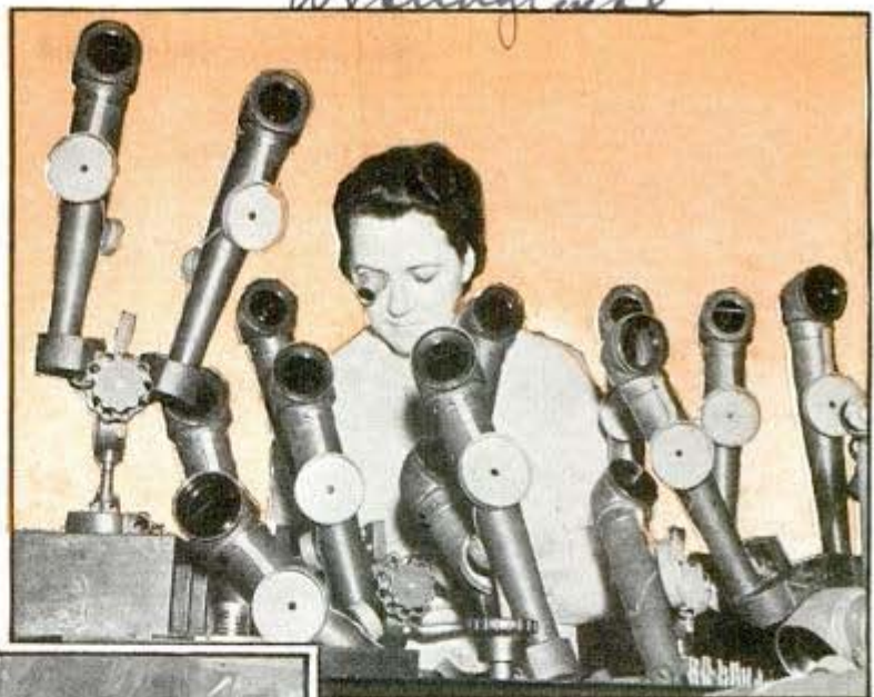
Checking instruments used in maintaining chronographs, which record bullet velocity. Optical glass is essential in making fire-control instruments
