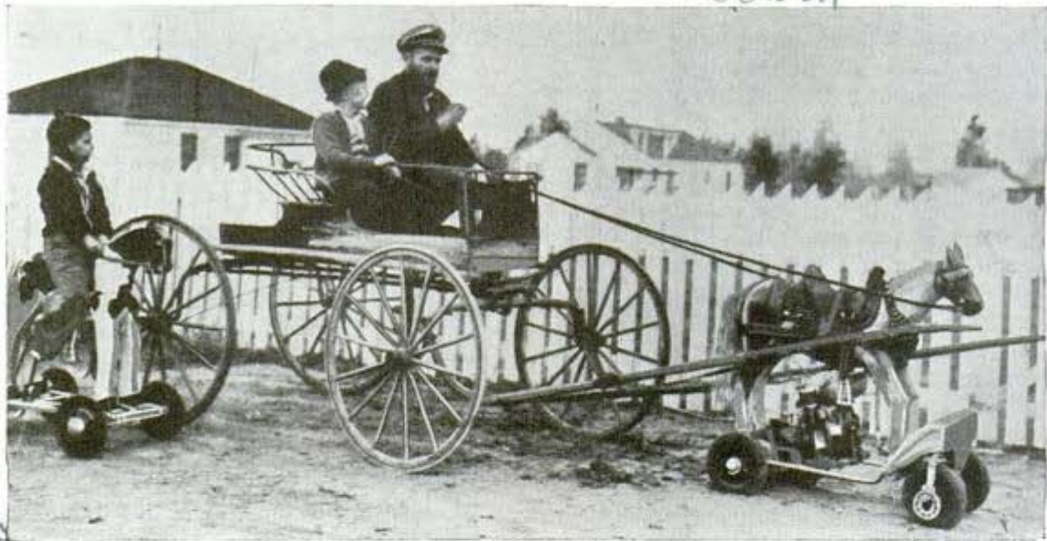
Hobbyhorse on wheels, controlled by reins and driven by a marine engine, pulls buggy or carries rider
