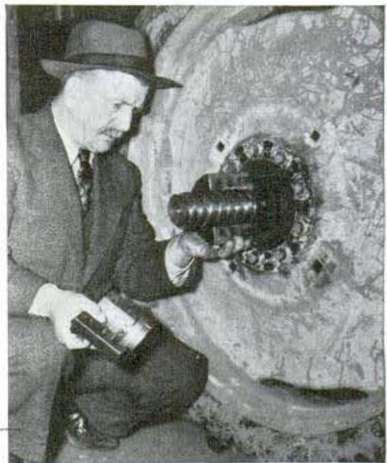
Here the inventor is holding half of the lock block against threaded axle to show how it clamps on hub
