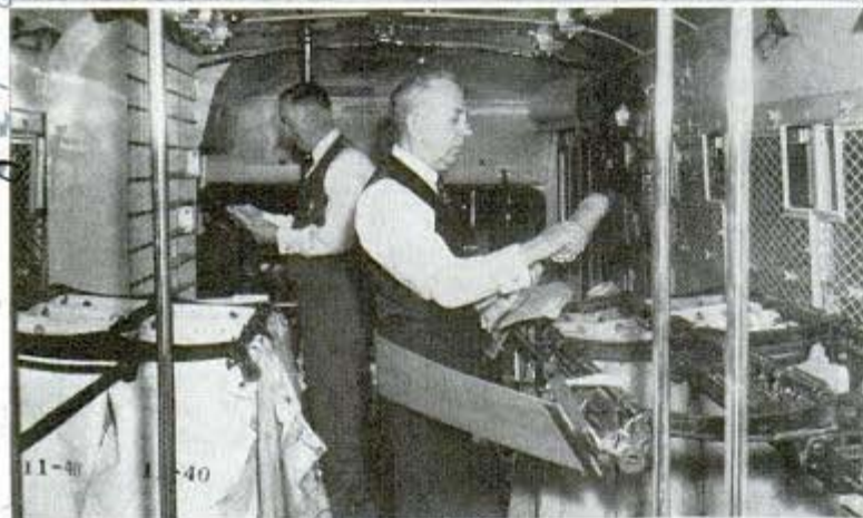
Resembling a passenger coach outside, but containing complete equipment for handling mail, highway bus will augment service to wayside stations
