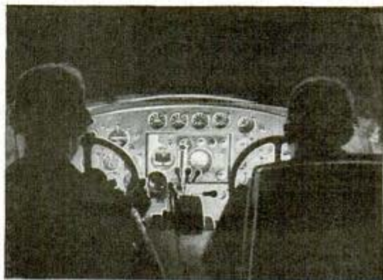
Battery of ultra-violet lamps making dials luminous can be seen at center of this Air Corps photo
