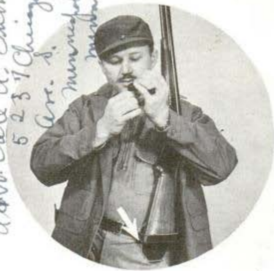
Gun rest, fastened to hunter's belt, relieves strain of carrying gun and keeps it handy for quick action
