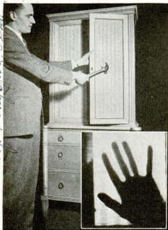
Inset in lower corner shows the translucent quality of the unbreakable plastic door panel
