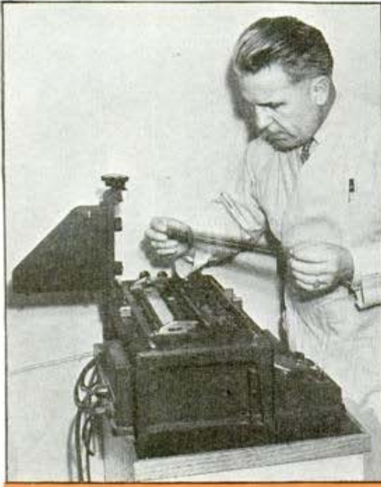
At right is a spectro-analytic film from which the expert can discern the elements in the substance studied; at left the film is being placed in projection machine
