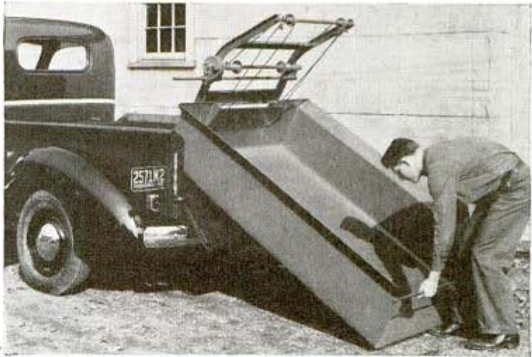
Truck operator ready to slide removable dump-bed into place. Frame at head supports crank and pulleys, one-man mechanism for tilting the body to dump the load
