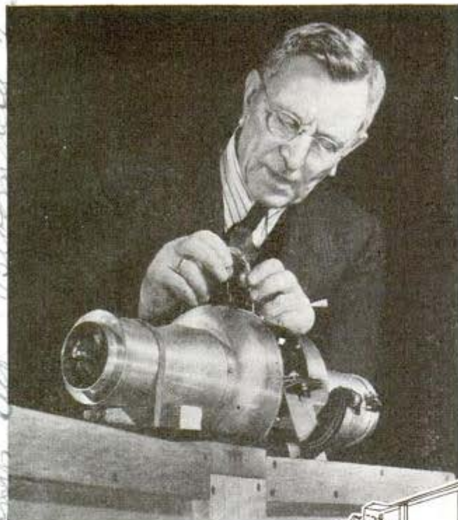
Left, adjusting the Klystron tube. Below, sketches showing how horn helps to direct or "shoot" the power beam so that small electric bulbs in its path will light up
