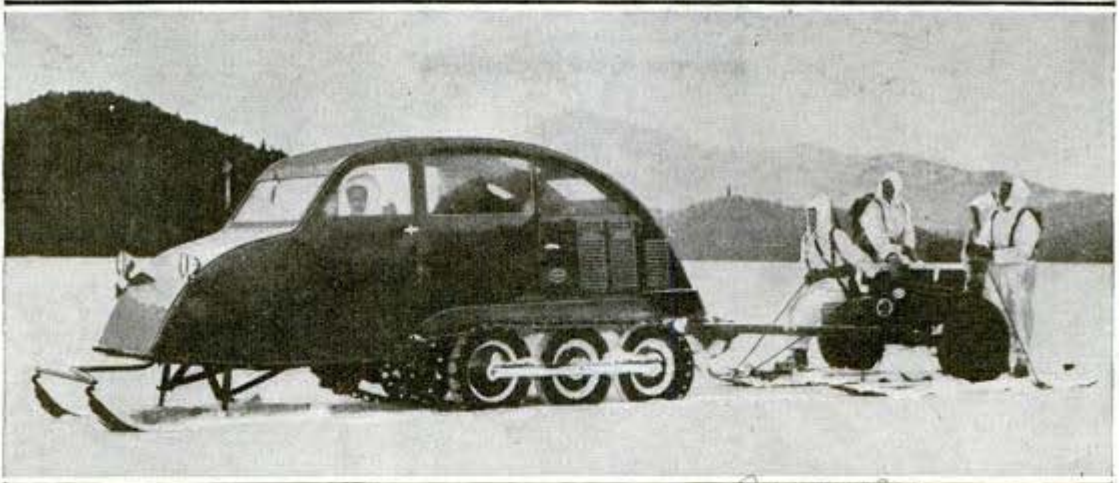
acme. Whiteclad ski troops of Sixteenth Infantry hauling an anti-tank gun over snow at Lake Placid, N. Y., use a "snowmobile" equipped with skis at the front end to tow the gun which also rides on skis
