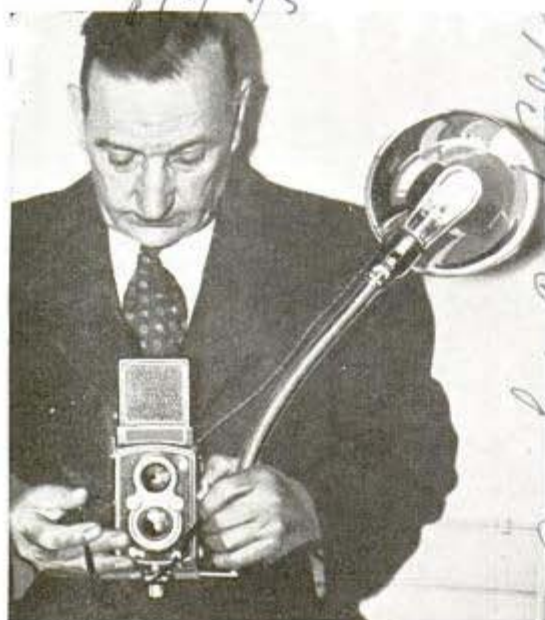
Extending from the flash gun on a flexible holder, bulb and reflector light scene from various angles
