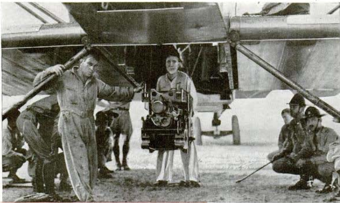
Above, loading a three-inch gun into a bombing plane. Below, a small part of air infantry's equipment that must be carried in plane. Included are motorcycles and life preservers. Each big transport can carry about two tons on normal hauls. Entire regiments, with equipment, can be transported easily by air
