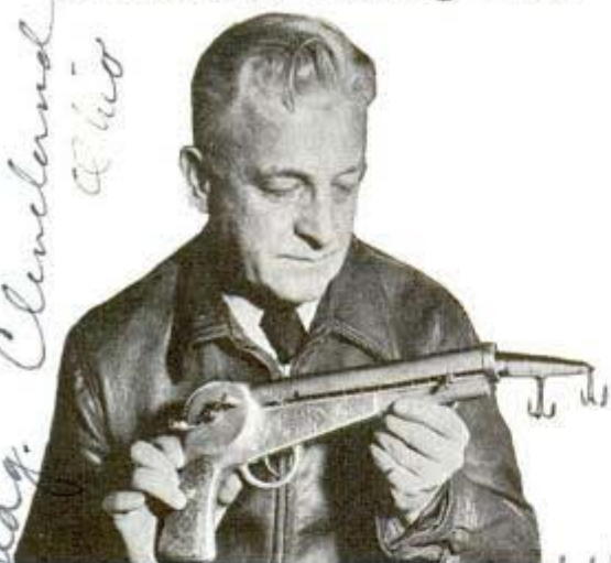
Better aim for inexperienced fishermen is possible with this line-casting gun that holds the reel
