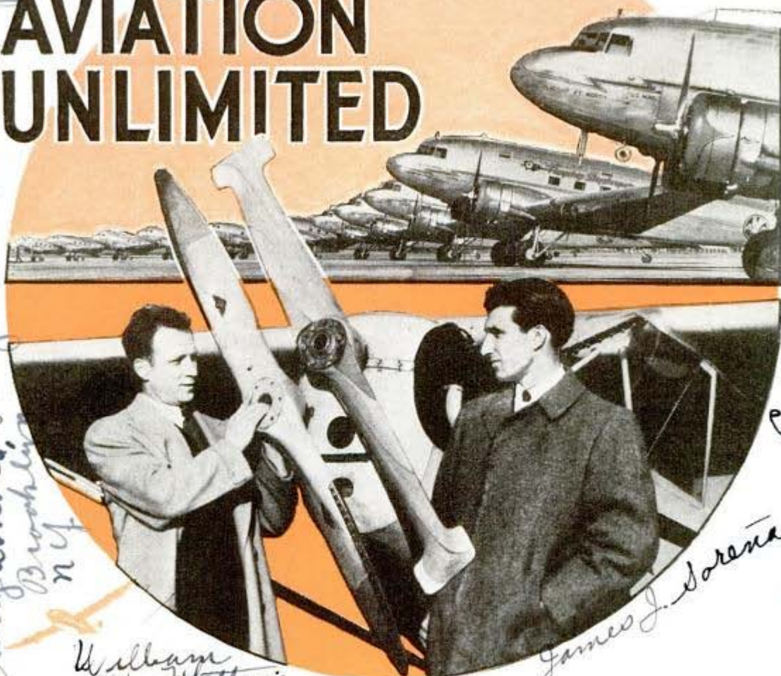
Comparing standard airplane propeller with "hammerhead" propeller which inventors claim is superior to those now in use. Above, group of big airliners at New York ready for a day's work
