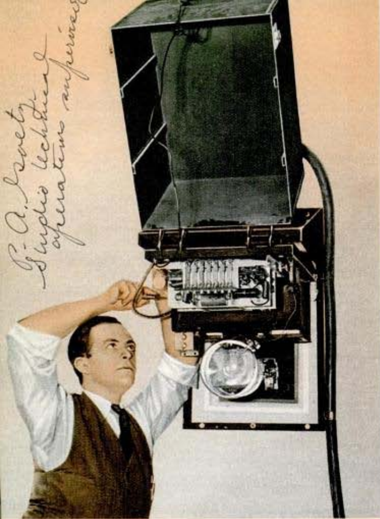
Above, making adjustments on CBS telecine camera in studio control booth. This camera is used to telecast motion pictures from films. Below, unusual view of antenna employed to get good results in television work.
