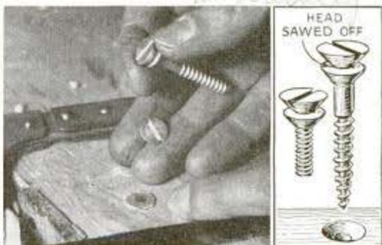
Drawing shows where slotted head is sawed off, leaving smooth-head screw or bolt permanently in place
