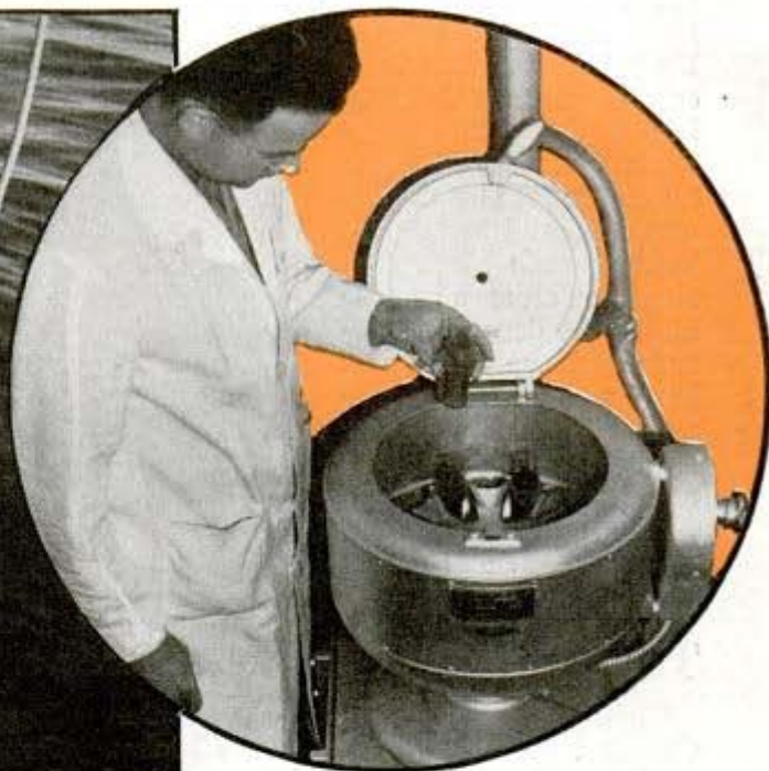
Left, corer being lowered to sample ocean bottom. Circle, centrifuge which whirls sea water at high speed to separate elements for analysis
