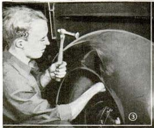
It is a simple job to remove small dents quickly with a dinging hammer and a dolly
