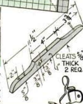
The simplicity of construction and assembly of this tilt-top table is apparent from these drawings. The top has two cleats on the underside, which pivot on a block glued to the pedestal. An elbow catch prevents the top from tipping when in horizontal position.
