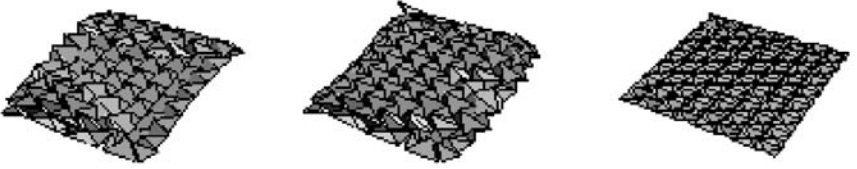
Figure 2. Typical configurations of the collapsed sheet. Two line defects in the overall down configuration are clearly visible in the two left-most configurations.
