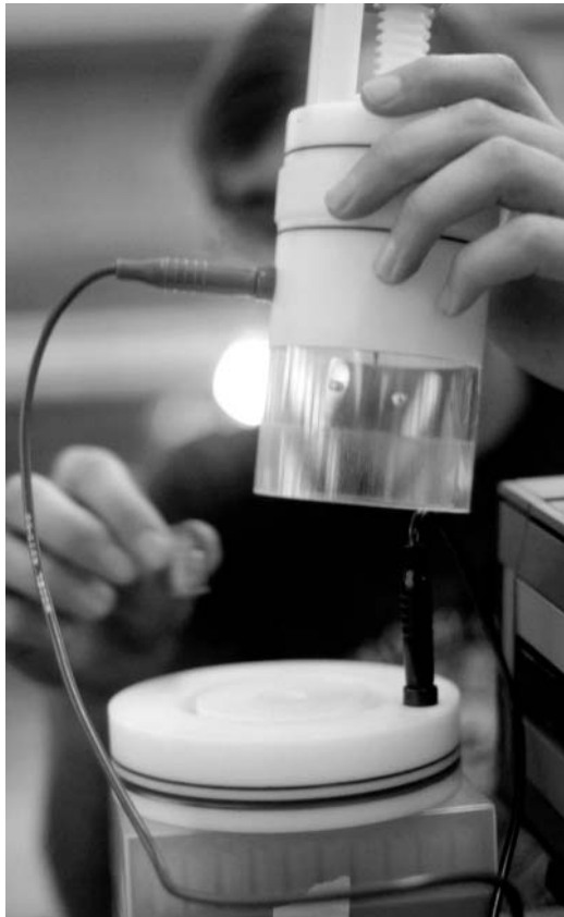
Fig. 10.3. Electroporation of fish eggs. Eggs (15–50) are placed in a DNA solution inside the cuvette and then placed between two electrodes to receive rapid pulses of high voltage.
