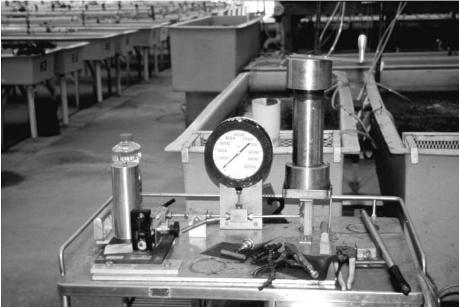
Fig. 3.1. Hydrostatic pressure chamber for inducing polyploidy. It is important to utilize a design that allows the bleeding off of all air to prevent the chamber from exploding and becoming a projectile. (Photograph by Rex Dunham.)
