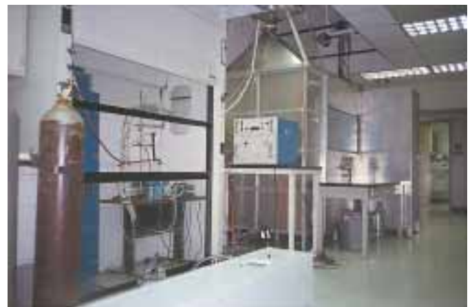
An exposure chamber for respiratory challenge studies. The subject is seated inside the metal chamber and gas or vapour is passed through a laminar flow wall into the chamber, inside which spirometry can be performed
