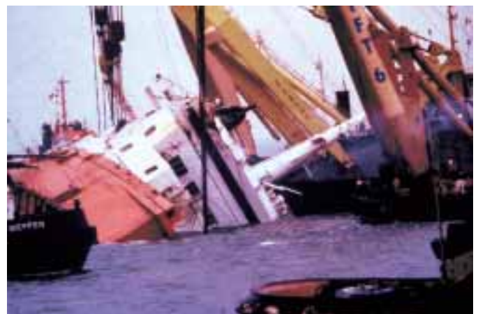
The Herald of Free Enterprise sank because no effective system was in place to ensure the bow doors were closed
