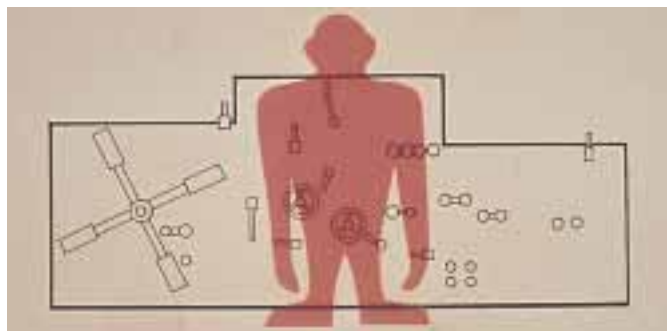
Arrangement of controls on a lathe and the “ideal” operator, who should have the following dimensions—4 feet 6 inches tall, shoulders 2 feet across, and an 8 foot arm span!
